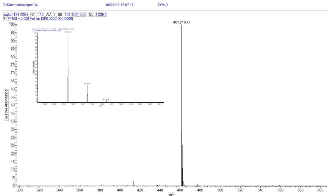
**Fig. S12** Positive-ion mode ESI mass spectrum of **5**. The inset shows the enlarged isotopic envelop for the  $[M+Na]^+$  species.
