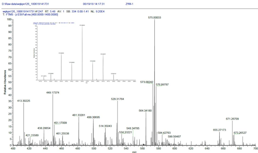
**Fig. S11** Negative-ion mode ESI mass spectrum of **2**. The inset shows the enlarged isotopic envelop for the  $[M-H]^-$  species.
