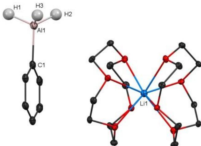
**Figure S2.4** Molecular structure of **4**, only hydrogen atoms attached to Al are shown, all other H atoms are omitted for clarity. Bond distances [ $\text{\AA}$ ] and angles [ $^\circ$ ] in **4** are: Al1-H1 1.54(5), Al1-H2 1.52(5), Al1-H3 1.45(4), Al1-C1 2.022(4); H1-Al1-H2 106(2), H1-Al1-H3 110(2), H1-Al1-C17 111(2), H2-Al1-H3 107(2), H2-Al1-C17-113(2), H3-Al1-C1 111(2). Hydrogen atoms at Al1 were located in the Fourier difference map.
