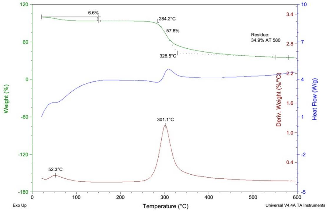
**Fig. S1.** The thermogravimetric analysis of CS
