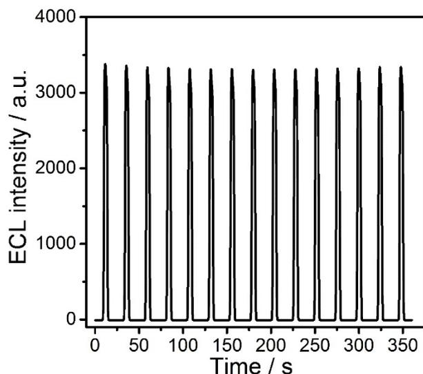
**Fig. S3** Stabilization of ECL signals from BSA/anchor DNA+swing arm:aptamer/RuSi NPs/CS/GCE with the successive incubation of the reaction solution consisting of 25000 particle/ $\mu\text{L}$  exosomes and Nb. BbvCI, and probe DNA-GOD conjugation.
