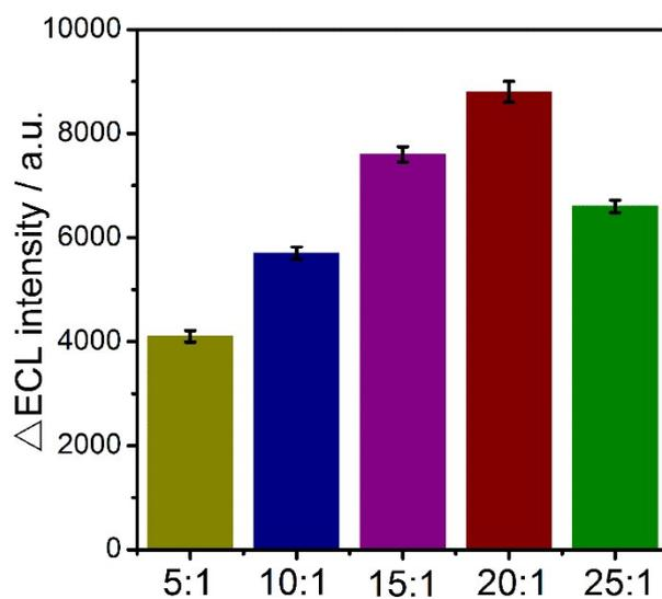
**Fig. S2** Bar graph of  $\Delta$ ECL intensity of ECL aptasensor with different concentration ratios between anchor DNA and swing arm.
