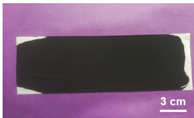
Fig. S7 Digital photographs of Co-NCNT coated separator prepared by blade coating method.
