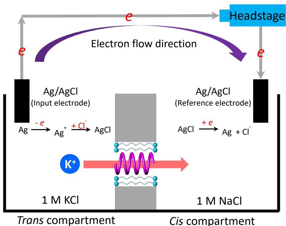
**Scheme S1.** Schematic illustration of the experimental setup for determining potassium transport selectivity ( $P_{\text{K}^+}/P_{\text{Na}^+}$ ). Redox reaction schemes on both Ag/AgCl electrodes were used to highlight the charge balance during  $\text{K}^+$  transport.
