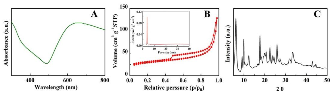
**Figure S2.** (A) The UV-vis spectrum of GNFs. (B) The  $\text{N}_2$  adsorption-desorption isotherms of MOFs (Inset: pore diameter of MOFs). (C) The XRD pattern of MOFs.
