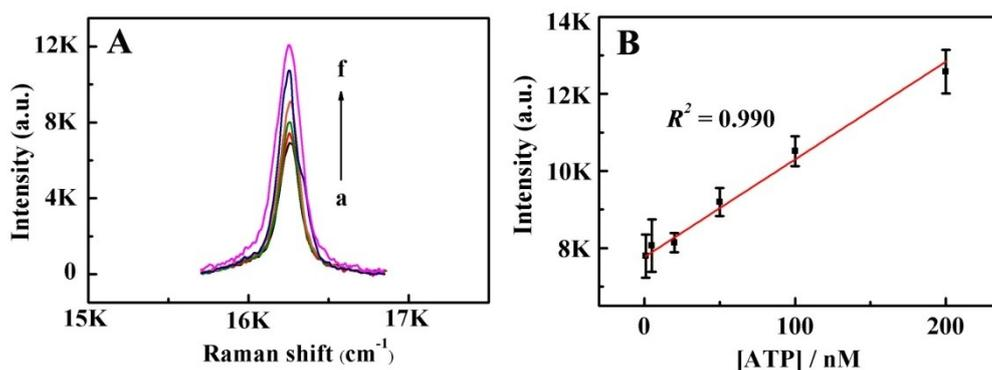
Figure S5. (A) The variation trend of Raman intensity of TB on GNFs without hairpin DNA (H1) with the increasing trend of the elevated concentration of ATP (nM) from a to f: (a) 1, (b) 5, (c) 20, (d) 50, (e) 100, (f) 200. (B) The calibration curve of TB Raman intensity on GNFs without hairpin DNA (H1) and ATP concentration (error bars = RSD,  $n = 3$ ).
