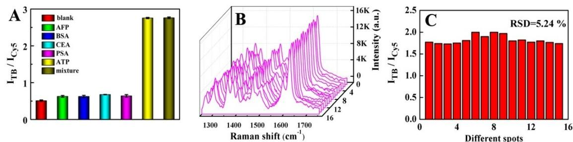
**Figure S6.** (A)  $I_{TB}/I_{Cys}$  values of the SERS sensor with series of interfering proteins, and the concentration of AFP, BSA, CEA and PSA are 10 ng/mL, ATP was 100 nM. (B) The SERS spectra and (C) the  $I_{TB}/I_{Cys}$  values of 15 different points after incubated with 100 nM ATP.
