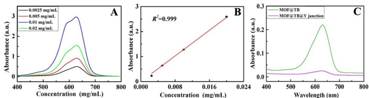
Figure S3. (A) The UV-vis absorption spectrums of TB standard solutions with different concentrations. (B) The standard curve of TB. (C) The UV-vis absorption spectrums of MOF@TB and MOF@TB@Y junction.
