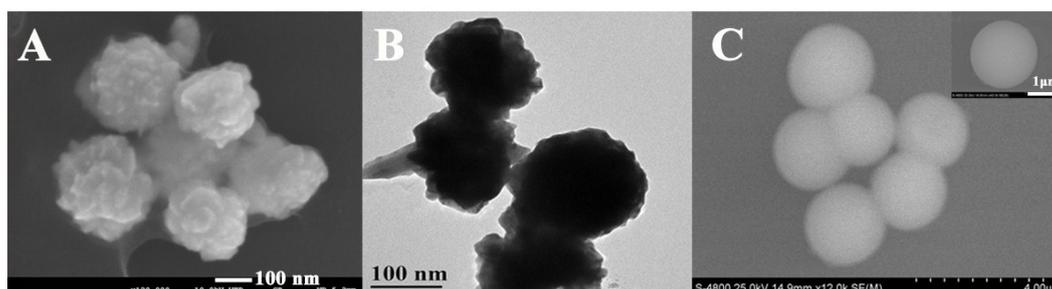
**Figure S1.** (A) SEM and (B) TEM of GNFs, SEM of (C) MOFs.
