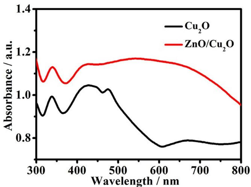
Fig. S3 UV-visible diffuse reflectance spectra (DRS) of  $\text{Cu}_2\text{O}$  and  $\text{Cu}_2\text{O}@\text{ZnO}$ .
