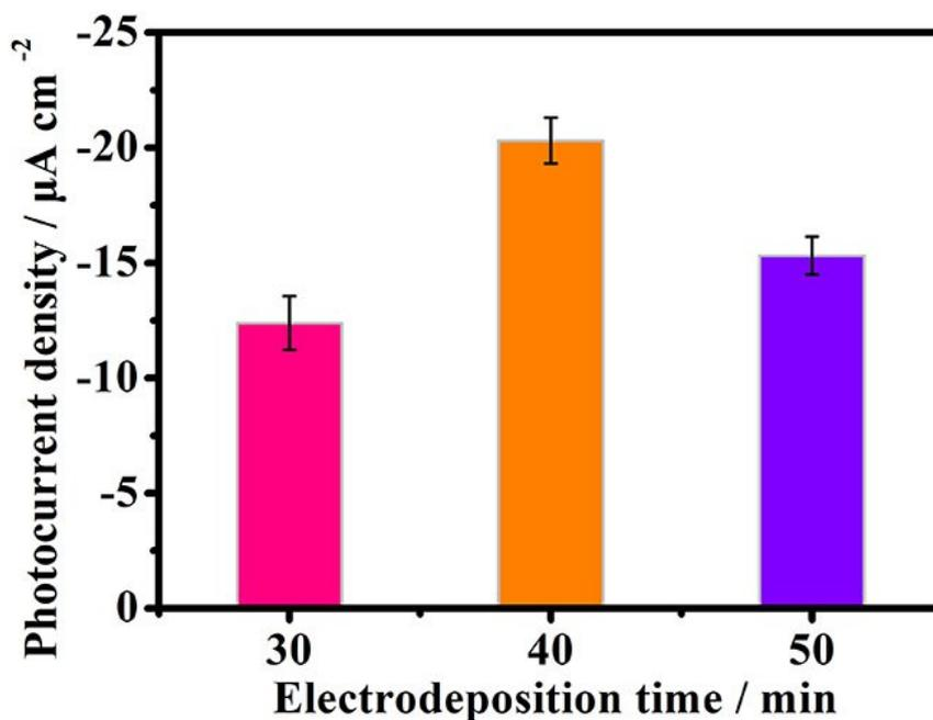
**Fig. S5** Optimization of PEC performance of  $\text{Cu}_2\text{O}$  with different electrodeposition time.
