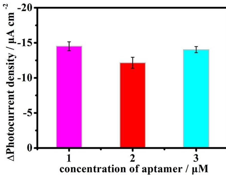
**Fig. S7** Optimization of PEC performance of Cu<sub>2</sub>O@ZnO/Au-aptamer with different concentrations of aptamer.
