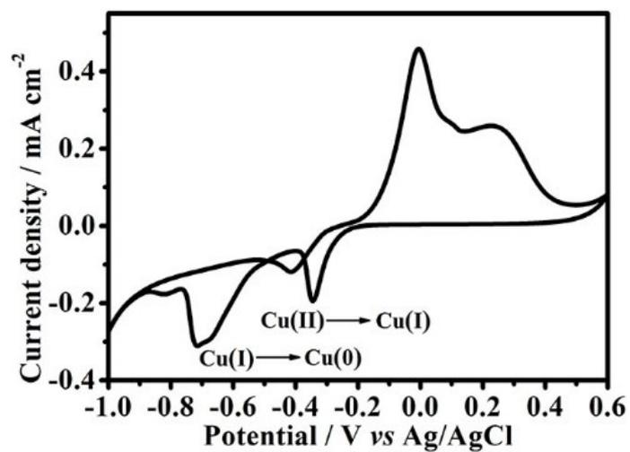
**Fig. S1** Cyclic voltammogram of FTO electrode in 1 mM copper citrate solution at a potential scan rate of 5 mV s<sup>-1</sup>.
