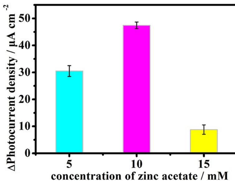
**Fig. S6** Optimization of PEC performance of  $\text{Cu}_2\text{O}@Z\text{nO}$  with different concentration of zinc acetate.
