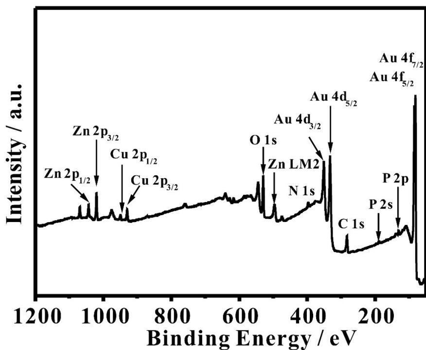
Fig. S4 XPS survey of  $\text{Cu}_2\text{O}@\text{ZnO}/\text{Au}$ -aptamer.
