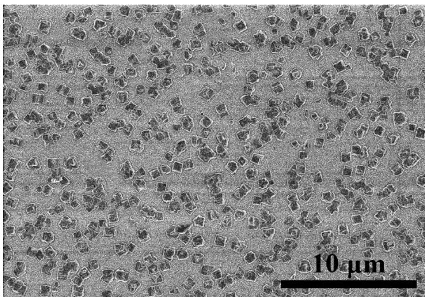
**Fig. S2** SEM image of Cu<sub>2</sub>O@ZnO in large scale.
