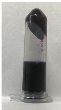
**Figure S14.** Image of precipitated  $4^{\bullet-}$  after addition of potassium persulfate to a 0.1 M solution of  $4^{2-}$ .
