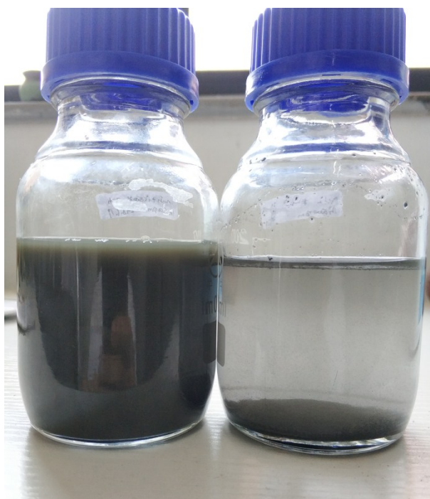
Figure S1. MoS 2 dispersions in water with (left) and without PyB-Na (right) right after shear mixing.
