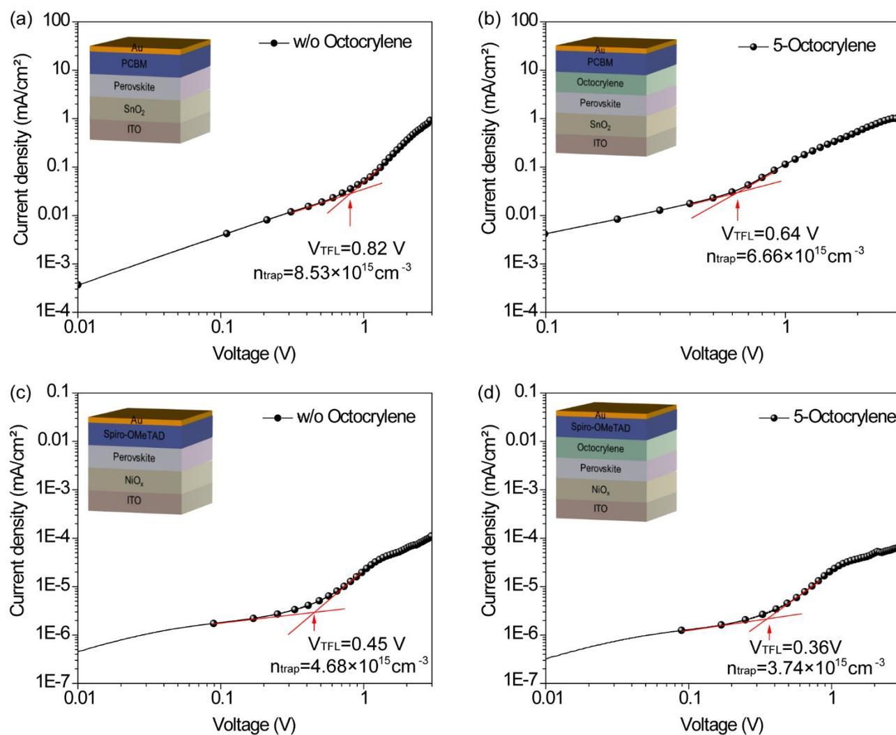
Fig.S3 Current–voltage curves and trap densities of (a and b) electron-only and (c and d) hole-only devices using the space-charge-limited current (SCLC) method (inset, device structure).
