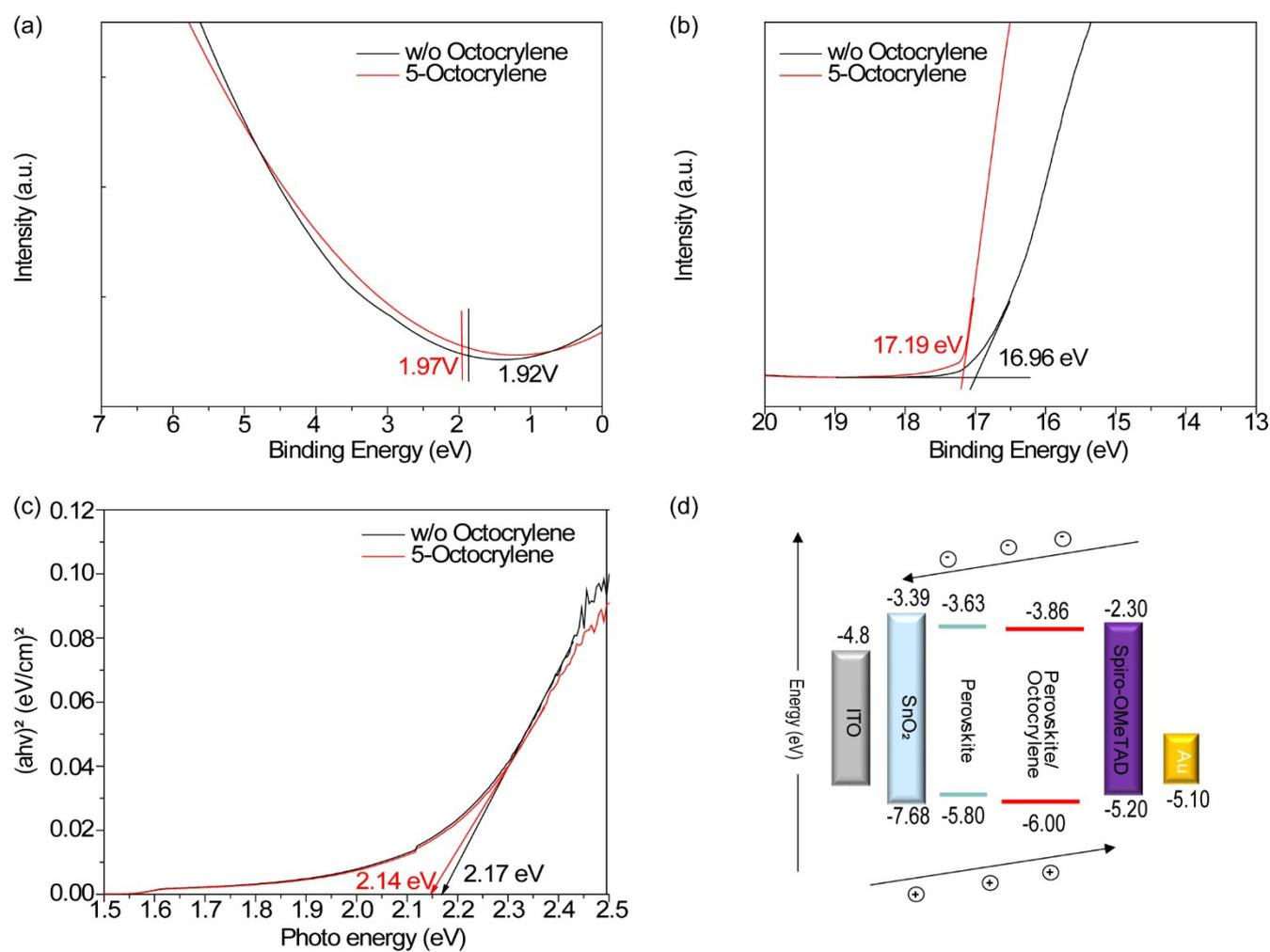
Fig.S4 (a) Valence band spectra. (b) The secondary electron cutoff (SEC) edge. (c) The band gap calculation using the Tauc plot. (d) Energy level diagram of the device.
