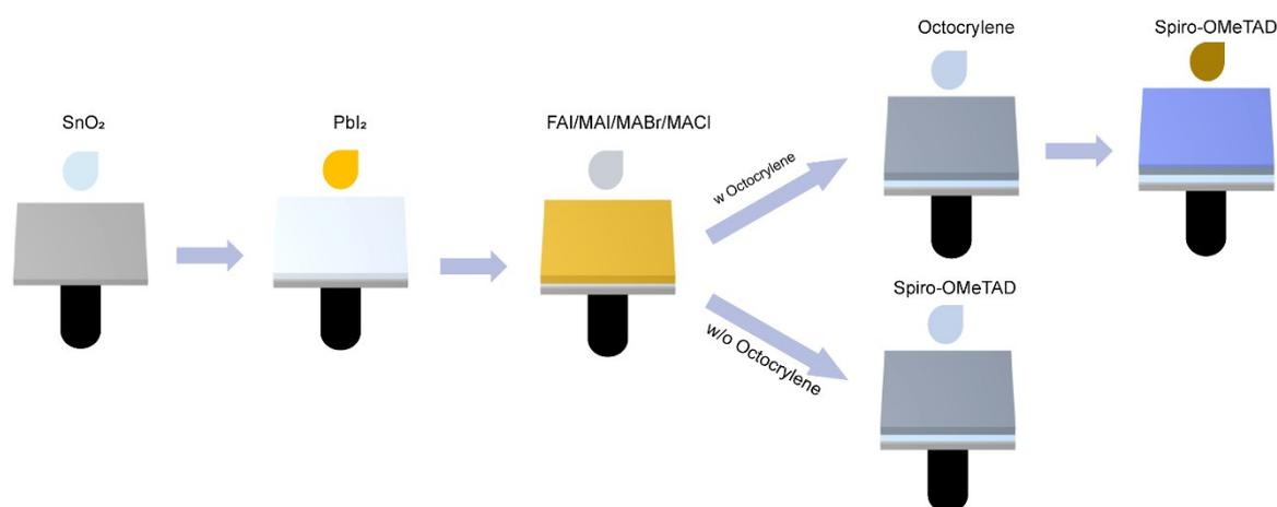
Fig. S1 Schematic representation of the manufacturing process for perovskite devices with and without octocrylene.
