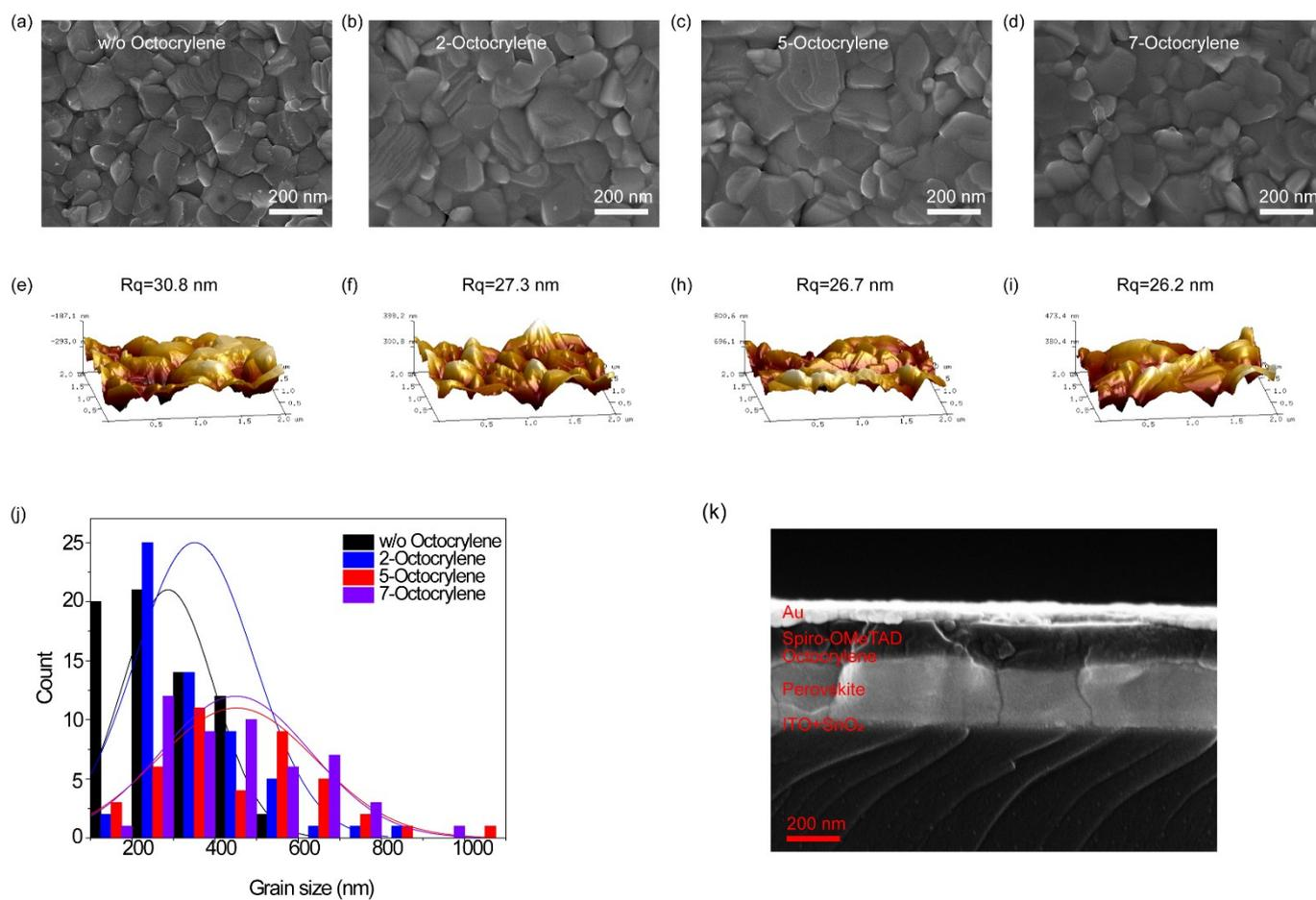
Fig. S2 The SEM and AFM images of the perovskite films (a) and (e) w/o octocrylene, (b) and (f) 2-Octocrylene, (c) and (h) 5-Octocrylene and (d) and (i) 7-Octocrylene. (j) Grain size distributions obtained from SEM images. (k) Cross-section image of the octocrylene device.
