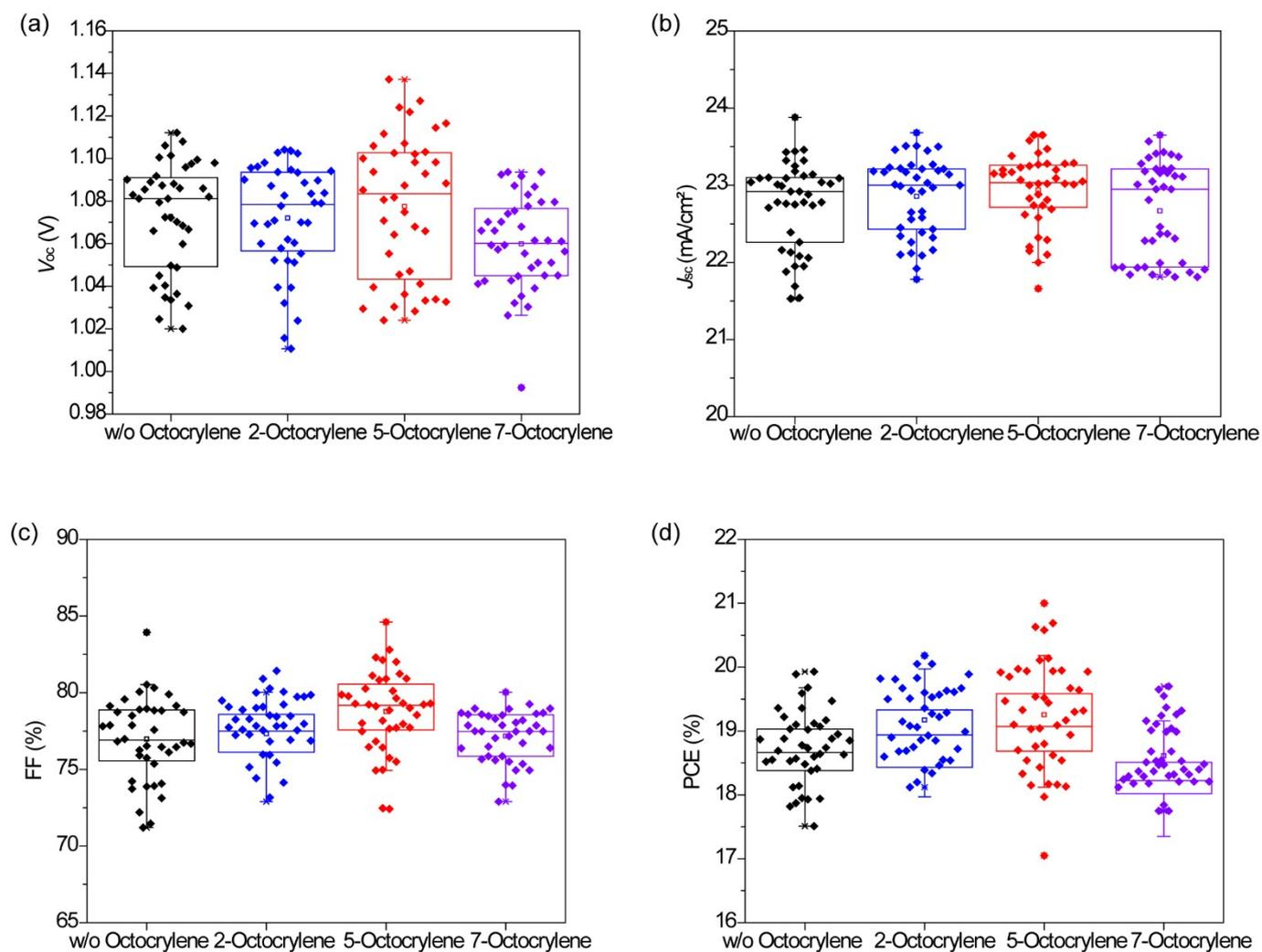
Fig.S5 Statistics on the distribution of (a)  $V_{oc}$ , (b)  $J_{sc}$ , (c) FF and (d) PCE of PSCs with different concentrations of octocrylene.
