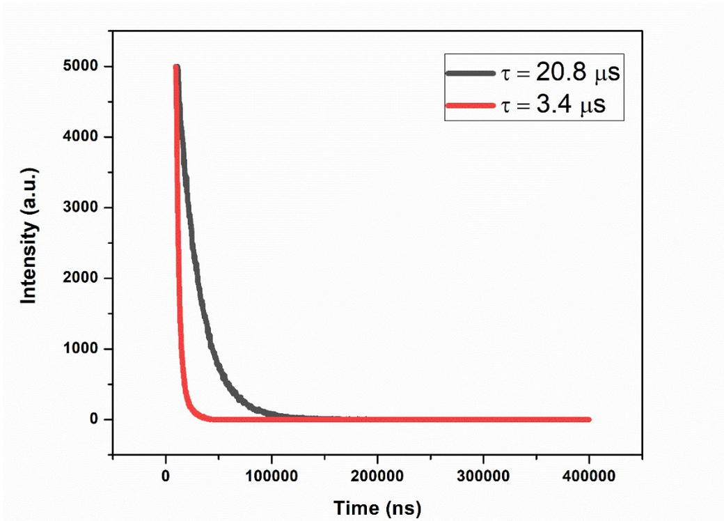
Figure S6. Luminescence decay spectra of **4** at 460 nm (black) and 550 nm (red).  $\lambda_{\text{ex}} = 360\text{nm}$ .
