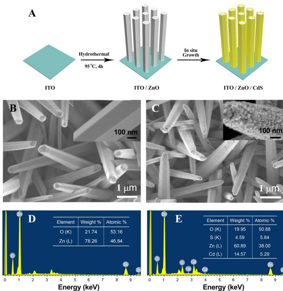
**Fig. S1** (A) Fabrication procedure of ITO/ZnO/CdS electrode. Top-view SEM images of (B) ITO/ZnO electrode and (C) ITO/ZnO/CdS electrode, and the insets are the high-magnification SEM images. EDS spectra and elemental percentages of (D) ITO/ZnO and (E) ITO/ZnO/CdS electrodes.
