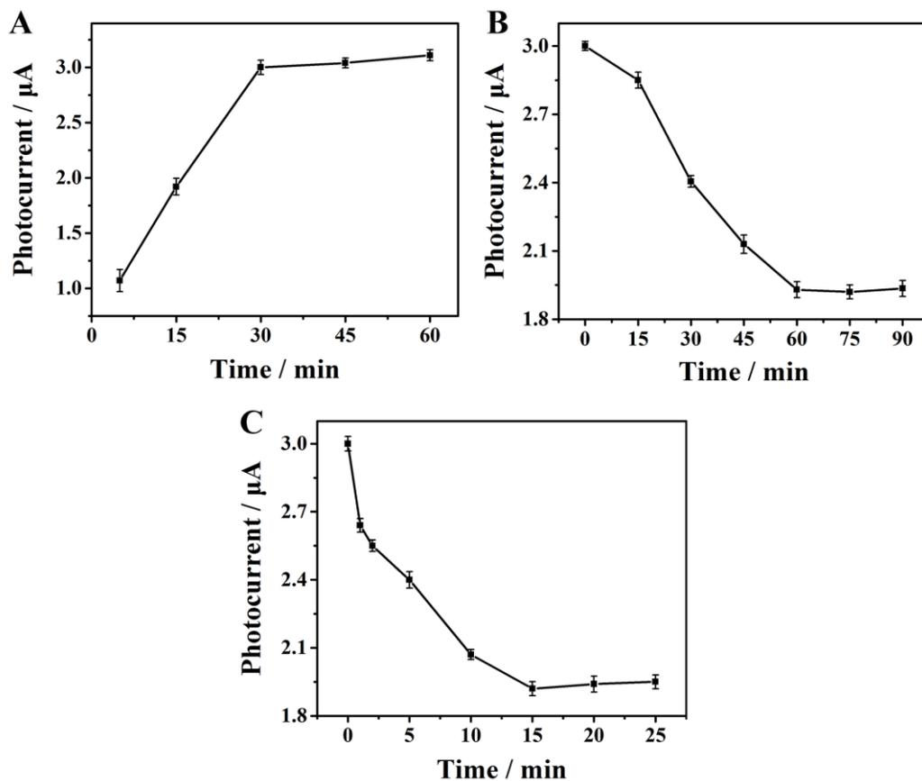
**Fig. S9** Optimization of the experimental conditions. The photocurrent versus (A) the *in-situ* deposition time of CdS (5, 15, 30, 45 and 60 min), (B) the reaction time of  $\lambda$ -Exo catalyzed digestion (0, 15, 30, 45, 60, 75 and 90 min), and (C) the catalytic reaction time of G-quadruplex/hemin (0, 1, 2, 5, 10, 15, 20 and 25 min).
