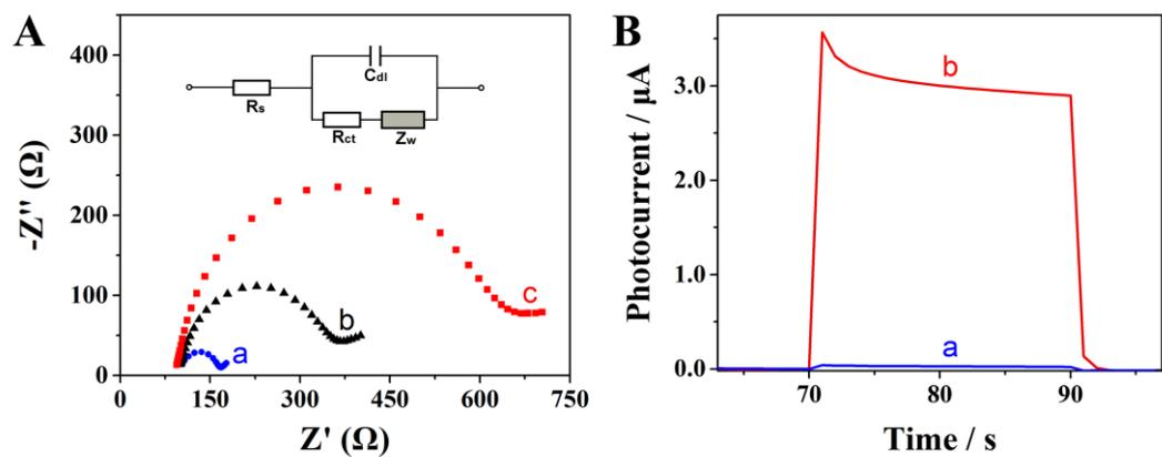
**Fig. S2** (A) EIS Nyquist plots of ITO electrodes at different modification stages: (a) bare ITO, (b) ITO/ZnO, and (c) ITO/ZnO/CdS; Inset: equivalent circuit. (B) Photocurrent response of (a) ITO/ZnO, and (b) ITO/ZnO/CdS electrodes in Tris-HCl buffer (pH 7.4) containing 10 mM  $H_2O_2$  and 1 mM dopamine.
