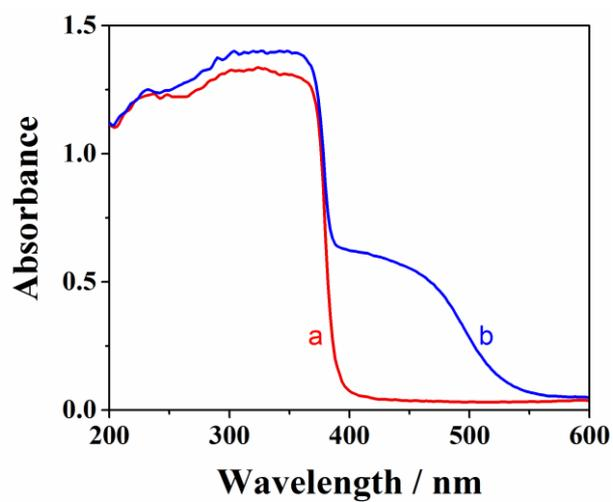
**Fig. S3** UV-vis absorption spectra of (a) ZnO and (b) ZnO/CdS heterostructure.
