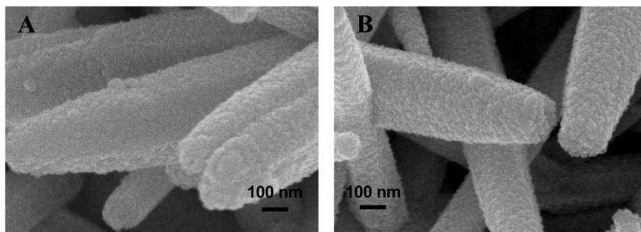
**Fig. S6** Top-view SEM images of ITO/ZnO/CdS electrode (A) before and (B) after photocurrent measurements.
