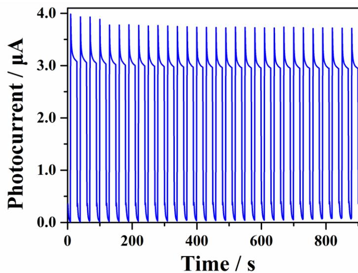
**Fig. S5** Photostability study: PEC response of ITO/ZnO/CdS electrode during 30 repeated on/off illumination cycles in the presence of 10 mM H<sub>2</sub>O<sub>2</sub> and 1 mM dopamine.
