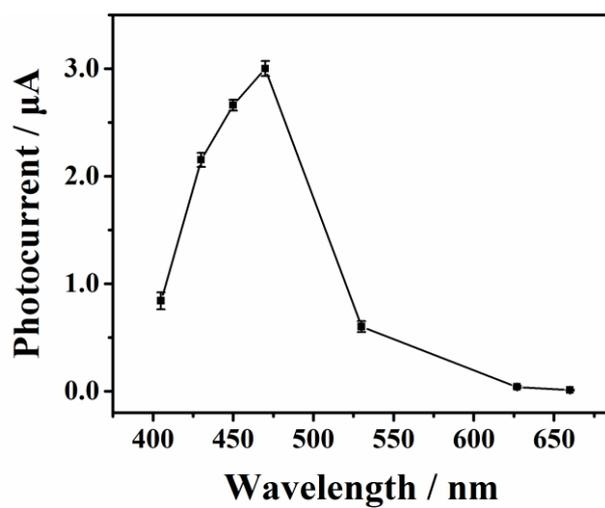
**Fig. S4** The photocurrent response of ITO/ZnO/CdS electrode in Tris-HCl buffer (pH 7.4) containing 10 mM H<sub>2</sub>O<sub>2</sub> and 1 mM dopamine using visible light source with different wavelengths: 405, 430, 450, 470, 530, 627 and 660 nm.
