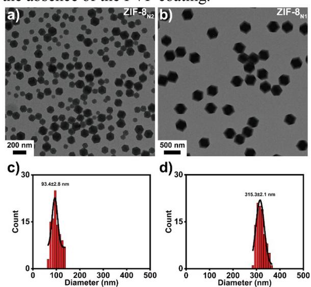
Figure S5. TEM images and size distributions of ZIF-8<sub>N2</sub> NPs (a, c) and ZIF-8<sub>N1</sub> NPs (b, d). Scale bar: 200 nm in (a), 500 nm in (b).
