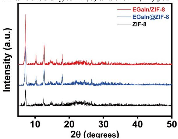
Figure S10. XRD patterns of LM@MOF composites and ZIF-8 nanoparticles.
