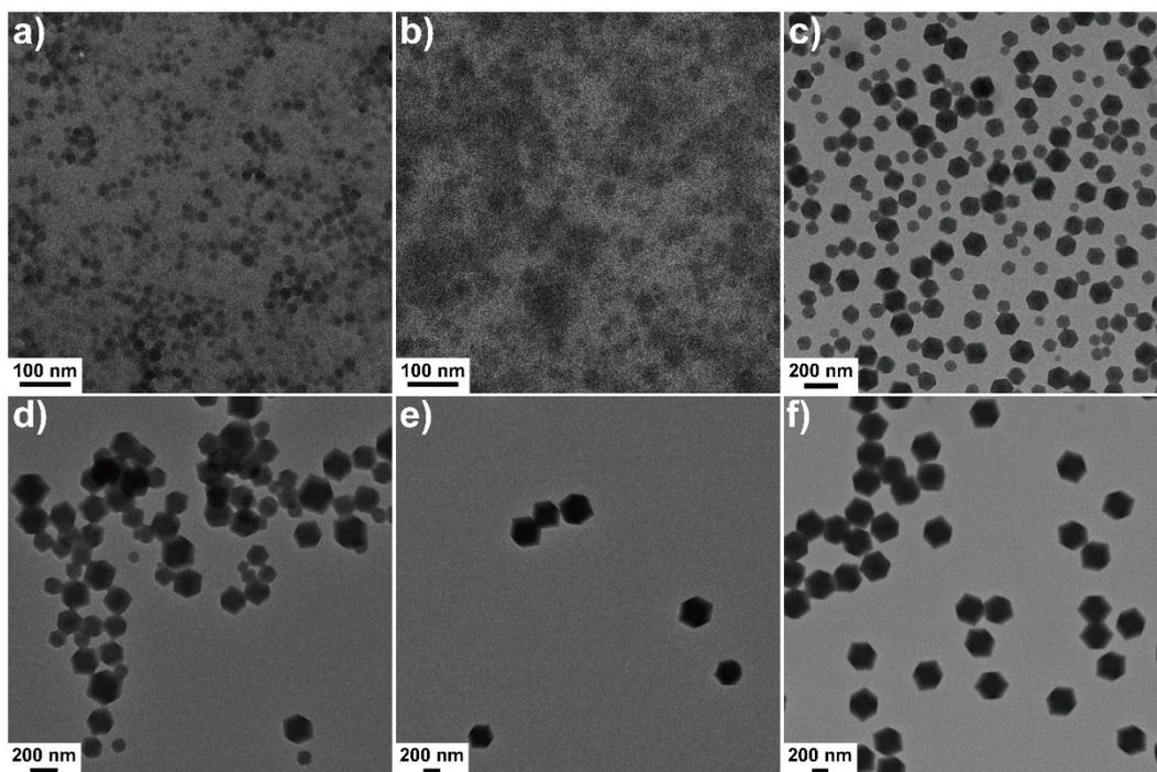
Figure S12. TEM images of ZIF-8 NPs with different L/M ratio: 4 (a), 2.7 (b), 2 (c), 1.5 (d), 1.2 (e), and 1 (f).
