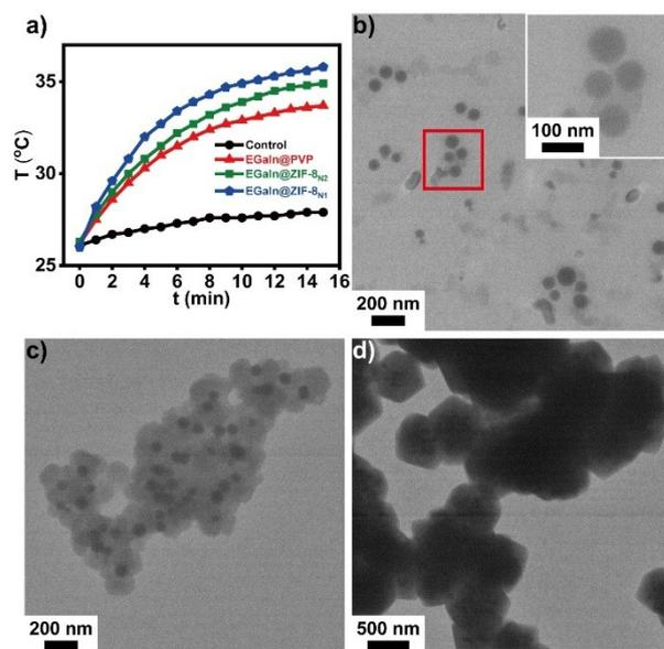
Figure S18. NIR light-activated photothermal conversion of LM@MOF composites. (a) Temperature increases of EGaIn NDs, EGaIn@ZIF-8<sub>N2</sub> NPs, EGaIn@ZIF-8<sub>N1</sub> NPs, and methanol upon light irradiation. (b-d) TEM images of EGaIn NDs (b), EGaIn@ZIF-8<sub>N2</sub> NPs (c), and EGaIn@ZIF-8<sub>N1</sub> NPs after light irradiation. Scale bar: 200 nm in (b) and (c), 100 nm in (b, inset), 500 nm in (d).
