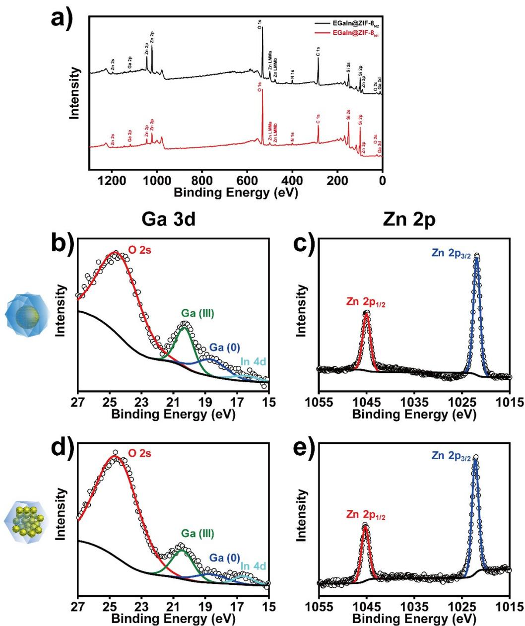
Figure S8. (a) XPS spectra of EGaIn@ZIF-8<sub>N2</sub> NPs and EGaIn@ZIF-8<sub>N1</sub> NPs. (b-e) Ga 3d and Zn 2p analysis of EGaIn@ZIF-8<sub>N2</sub> NPs (b-c) and EGaIn@ZIF-8<sub>N1</sub> NPs (d-e).
