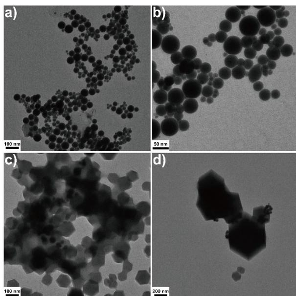
Figure S4. TEM images of bare EGaIn NDs (a-b) and their ZIF-8 composites with different L/M ratio N2 (c) and N1 (d). EGaIn NDs cannot be encapsulated in ZIF-8 in the absence of the PVP coating.
