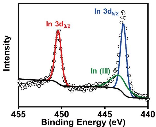
Figure S9. In 3d region of EGaIn@PVP NDs. The two In  $3d_{3/2, 5/2}$  peaks at 450.4 and 442.9 eV belong to In (0) and the In (III) peak at 443.5 eV is from  $\text{In}^{3+}$ .
