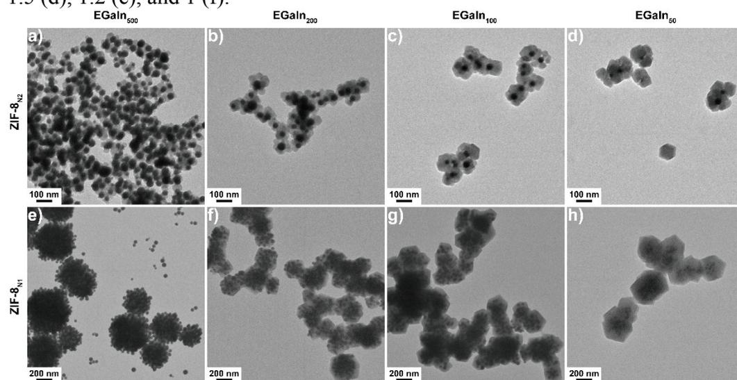
Figure S13. TEM images of EGaIn@ZIF-8 NPs synthesized using different amount of EGaIn (indicated by volume 500, 200, 100, and 50  $\mu$ L) and L/M ratio (indicated by N2 and N1).
