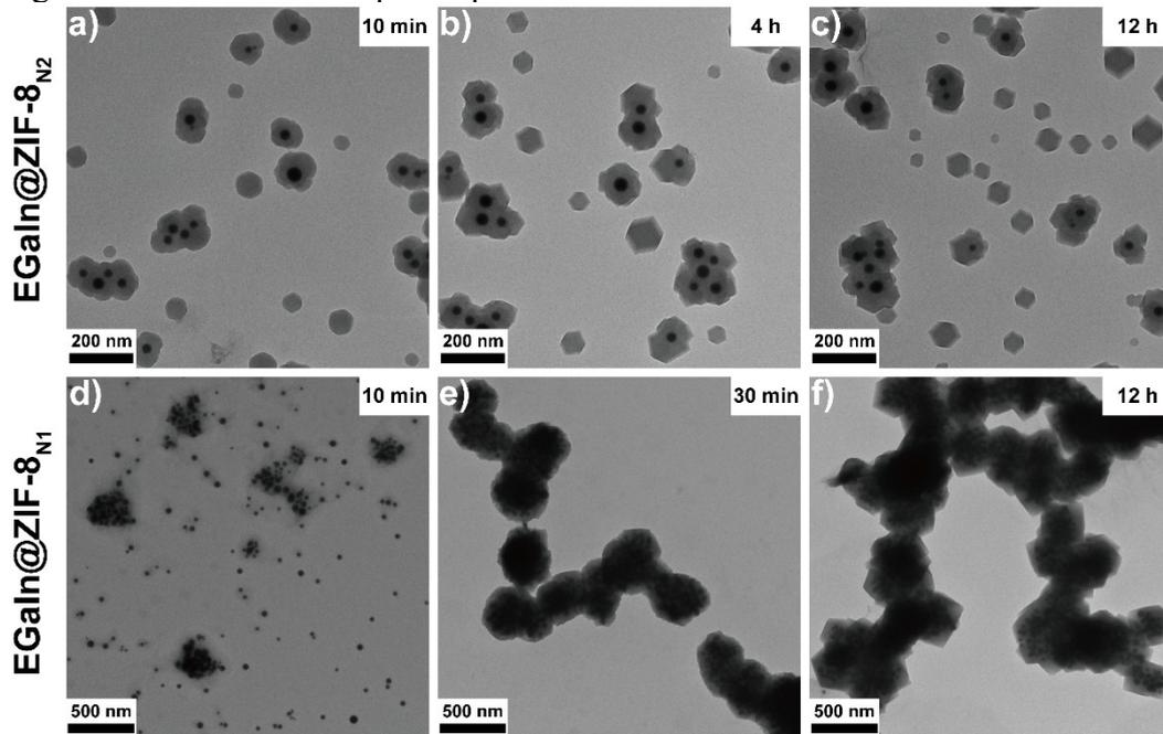
Figure S16. Structural evolution of EGaIn@ZIF-8 NPs. Time-dependent TEM images of EGaIn@ZIF-8<sub>N2</sub> NPs (a-c) and EGaIn@ZIF-8<sub>N1</sub> NPs (d-f). Scale bar: 200 nm in (a-c). 500 nm in (d-f).
