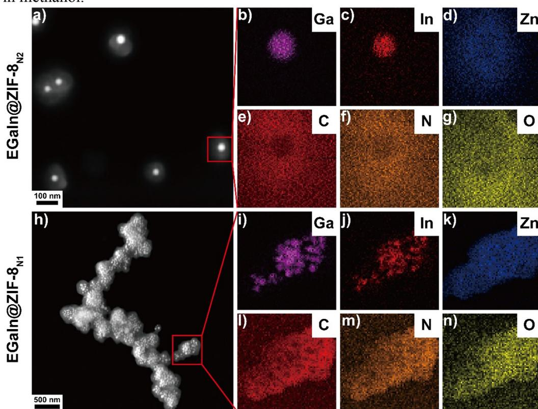
Figure S7. HAADF-STEM images and EDX mapping of EGaIn@ZIF-8<sub>N2</sub> NPs (a-g) and EGaIn@ZIF-8<sub>N1</sub> NPs (h-n). Scale bar: 100 nm in (a), 500 nm in (h).
