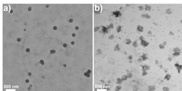
Figure S14. TEM images of ZIF-8<sub>N2</sub> clusters (a) and ZIF-8<sub>N1</sub> clusters (b) after 2 min reaction. Scale bar: 500 nm in (a-b).
