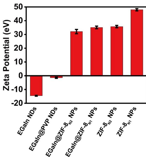
Figure S6. Zeta potential analysis. EGaIn NDs refers to bare EGaIn NDs synthesized in methanol.
