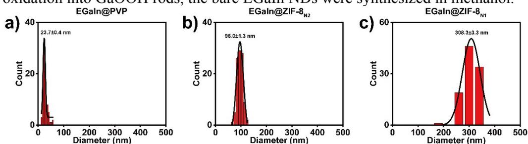
Figure S2. TEM size distributions of (a) EGaIn@PVP NDs, (b) EGaIn@ZIF-8<sub>N2</sub> NPs, and (c) EGaIn@ZIF-8<sub>N1</sub> NPs.
