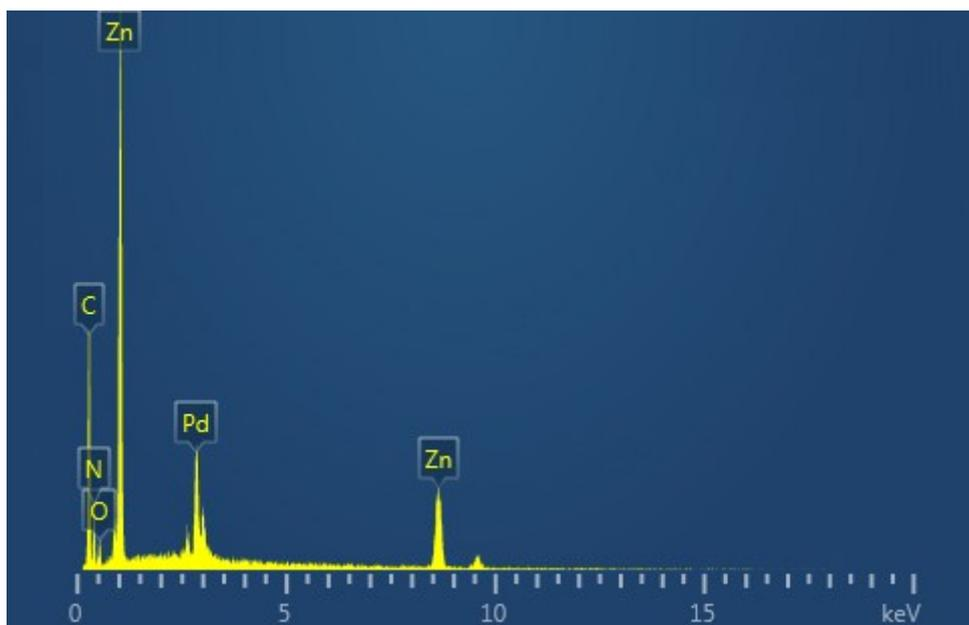
**Figure S3** Element analysis of Pd/NMC.
