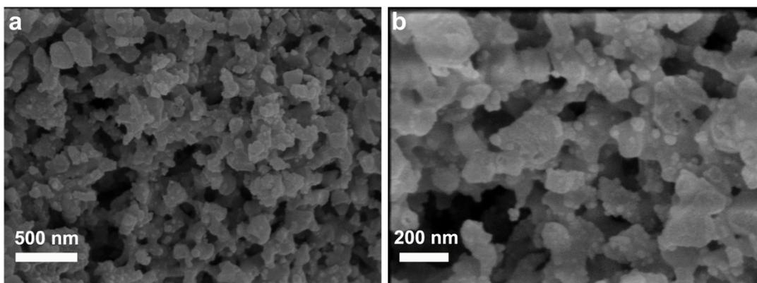
**Figure S6** SEM images of Pd/NMC after 6 cycles.
