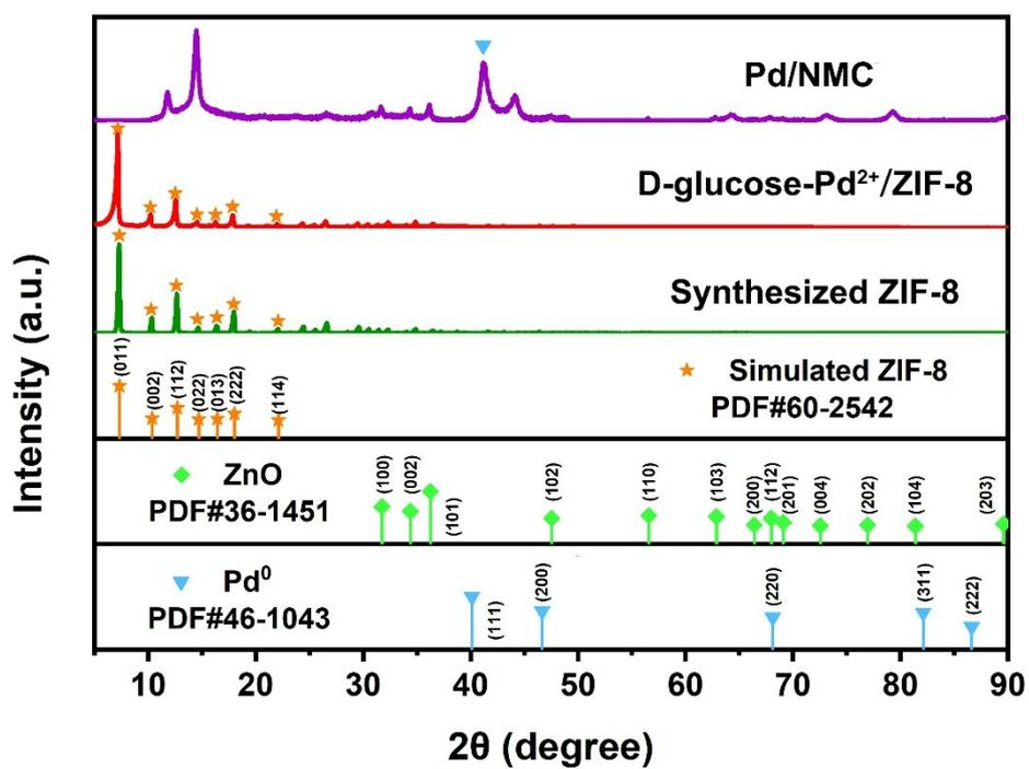
**Figure S2** XRD patterns of Pd<sup>0</sup> (PDF#46-1043), ZnO (PDF#36-1451), simulated ZIF-8 (PDF#60-2542), synthesized ZIF-8, D-glucose-Pd<sup>2+</sup>/ZIF-8 and Pd/NMC.
