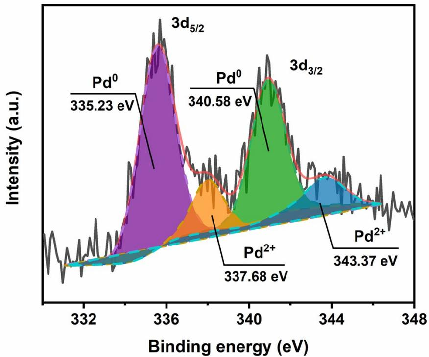
Figure S5 Pd 3d XPS spectrum of Pd/NMC.
