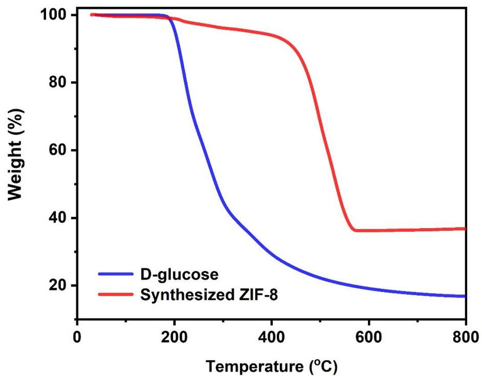
Figure S1 TGA analyses of synthesized ZIF-8 and D-glucose.
