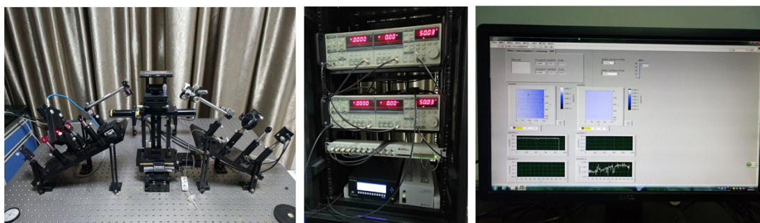
Fig. S1. Photographs of homemade OIRD setup. From left to right: optical components; lock-in amplifiers and PEM controller; software interface.
