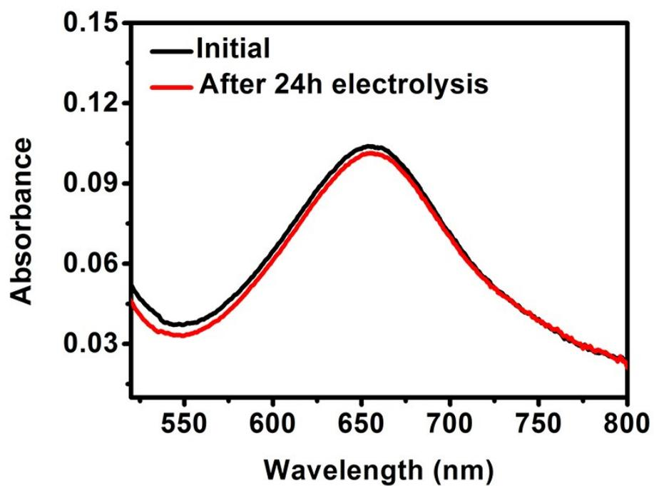
**Fig. S14.** UV-Vis absorption spectra of the electrolytes stained with indophenol indicator at  $-0.60$  V after electrolysis for 2 h with the initial Bi ND/CP and the Bi ND/CP after 24-h electrolysis.
