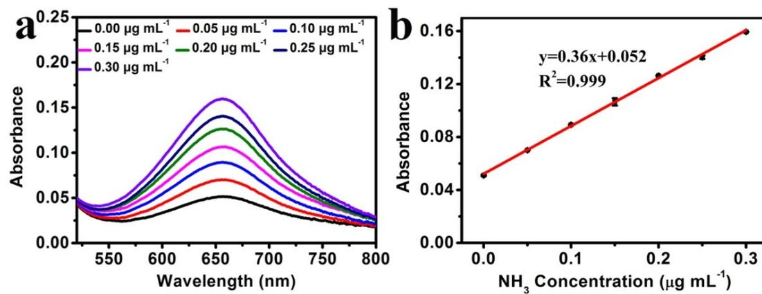
**Fig. S1.** (a) UV-Vis absorption curves of indophenol assays with  $\text{NH}_3$  concentrations after incubated for 2 h at room temperature in 0.1 M HCl. (b) Calibration curve used for estimation of  $\text{NH}_3$ .
