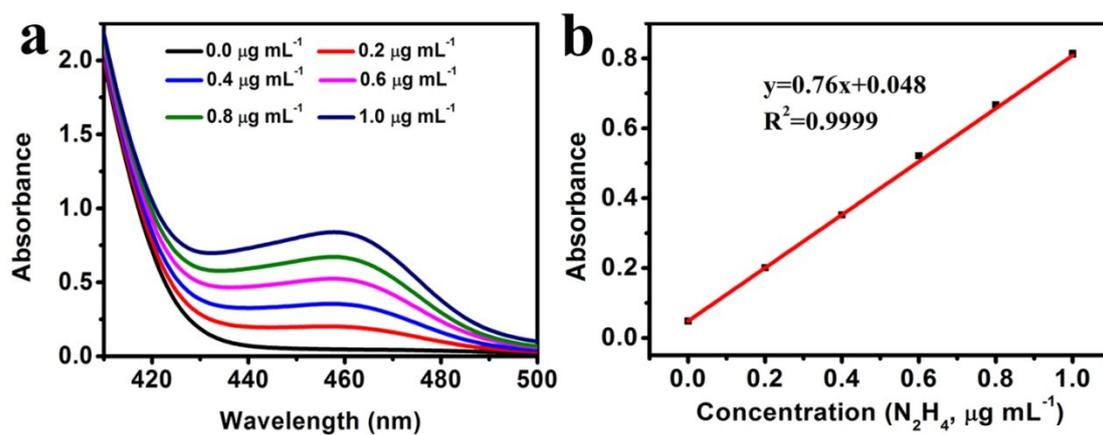
**Fig. S2.** (a) UV-Vis absorption spectra of  $N_2H_4$  concentrations after incubated for 20 min at room temperature. (b) Calibration curve used for calculation of  $N_2H_4$  concentrations.
