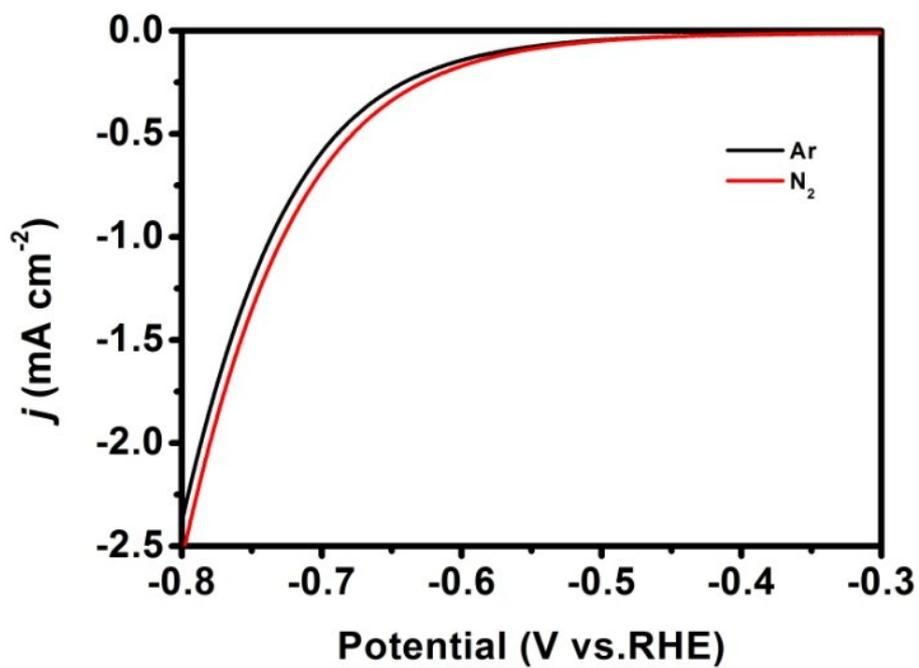
**Fig. S3.** LSV curves of Bi ND/CP in N<sub>2</sub>-saturated and Ar-saturated 0.1 M HCl electrolyte at a scan rate of 5 mV s<sup>-1</sup>.
