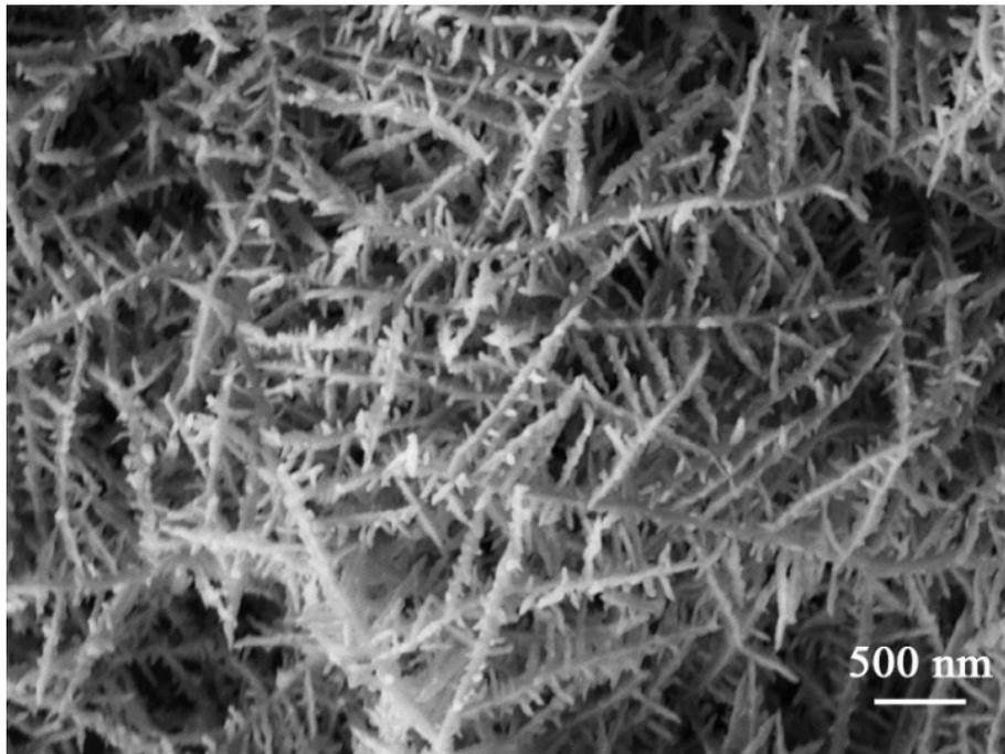
**Fig. S16.** SEM image for Bi ND after stability test.
