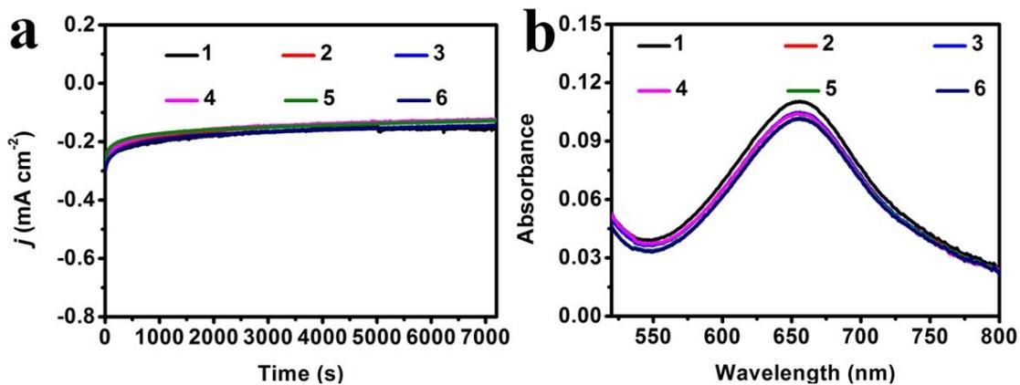
**Fig. S12.** (a) Time-dependent current density curves of Bi ND/CP electrode at -0.60 V over 6 cycles. (b) UV-Vis absorption spectra of the electrolytes stained with indophenol indicator after 2 h NRR electrolysis at -0.60 V over 6 cycles.
