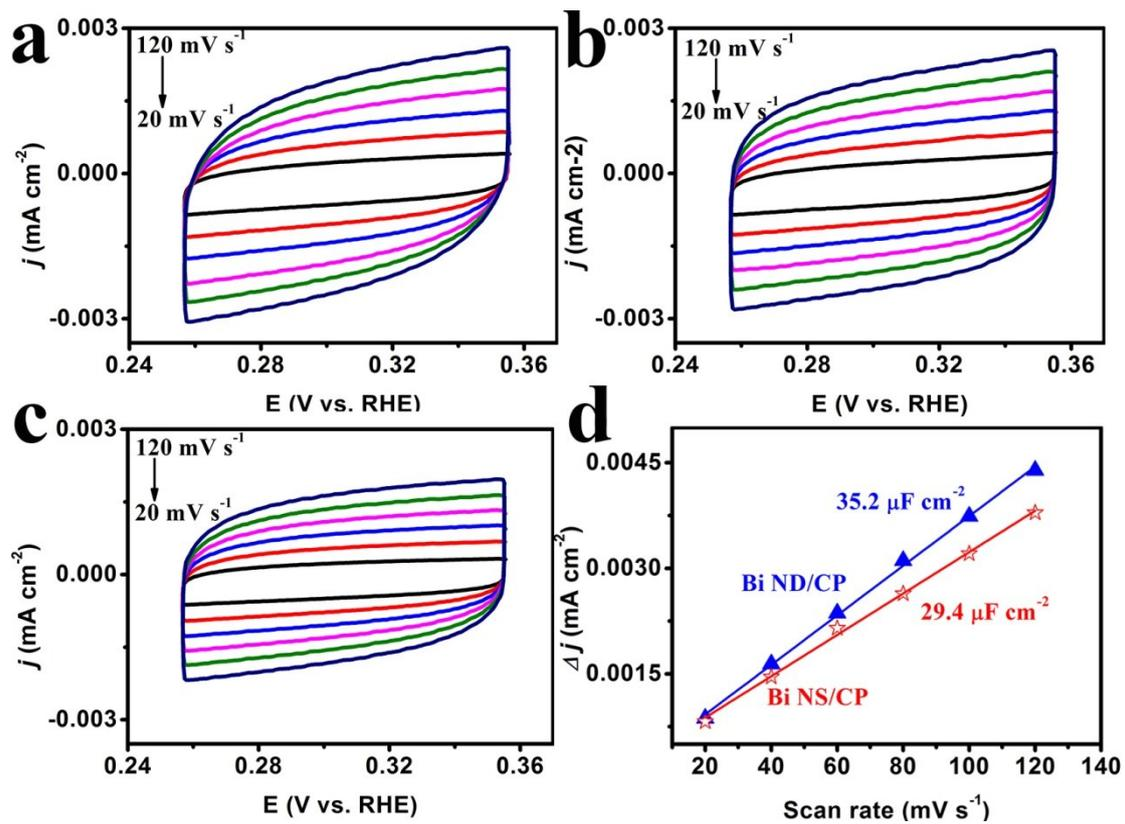
**Fig. S8.** CVs of (a) Bi ND/CP, (b) Bi NS/CP and (c) bare CP in the non-faradaic capacitance current range with various scan rates (20-120 mV s<sup>-1</sup>) in the region of 0.256 to 0.356 V vs. RHE. (d) Corresponding capacitive currents at 0.306 V vs. RHE as a function of scan rates for Bi ND/CP and Bi NS/CP.
