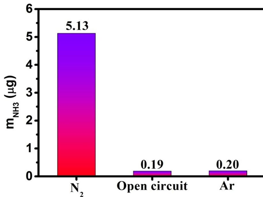
**Fig. S11.** Comparison of amount of NH<sub>3</sub> generated under different conditions.
