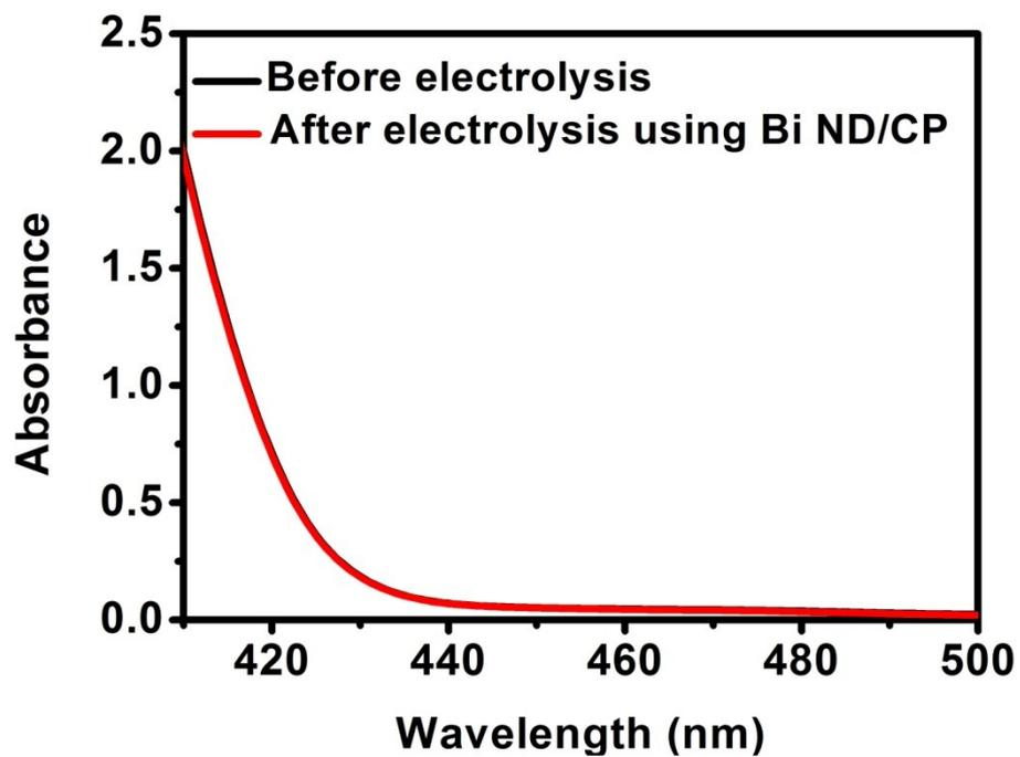
**Fig. S4.** UV-Vis absorption curves of the electrolytes treated with the method of Watt and Crisp for 20 min after NRR at a series of potentials.
