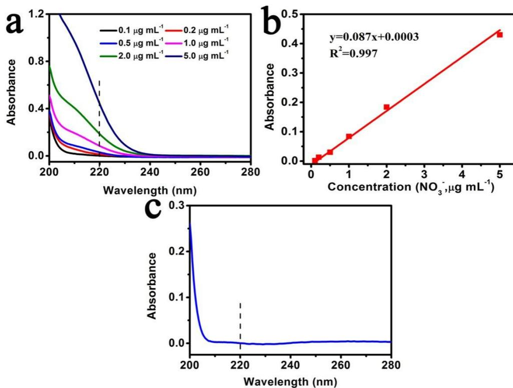
**Fig. S10.** (a) UV-Vis absorption spectra of different concentrations of  $\text{LiNO}_3$ . (b) Calibration curve used for calculating the concentration of  $\text{NO}_3^-$ . (c) UV-Vis absorption spectra for the determination of  $\text{NO}_3^-$  in the supernatant of the washed dendritic Bi.
