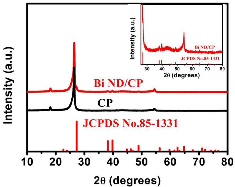
Fig. S15. XRD patterns for Bi ND/CP and CP after stability test.
