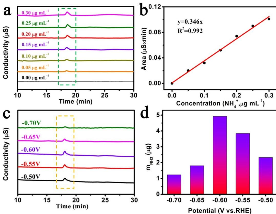
**Fig. S9.** (a) Ion chromatograms of  $\text{NH}_4\text{Cl}$  with various concentrations in 0.1 M HCl. (b) Calibration curve used for estimation of  $\text{NH}_3$ . (c) Curves of ion chromatography of Bi ND/CP after NRR electrolysis at different potentials for 2 h. (d)  $m_{\text{NH}_3}$  of Bi ND/CP for the  $\text{N}_2$  reduction at a series of potentials attained by ion chromatography.
