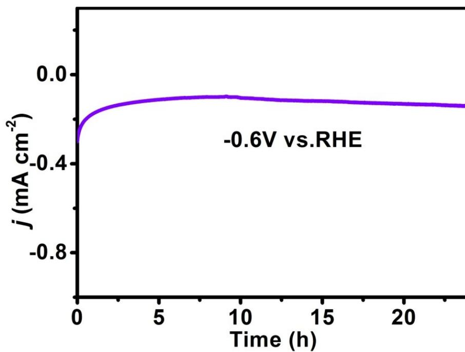
**Fig. S13.** Time-dependent current density curve for Bi ND/CP at  $-0.60$  V for 24 h.
