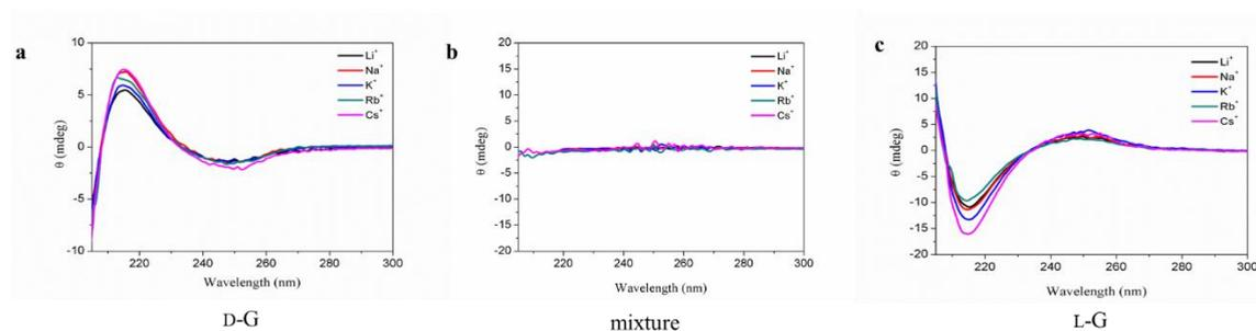
**Figure S4.** CD spectra. (a) D-G exhibited positive peaks at the wavelength of 215 nm. (b) Mixture at the rate of 1:1 showed no peaks. (c) L-G exhibited negative peaks at the wavelength of 215 nm. D-G and L-G showed opposite chirality.
