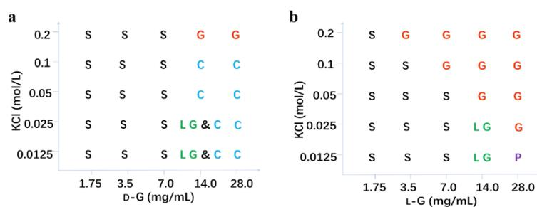
**Figure S7.** Phase diagram of the hydrogel formation ability at different concentrations of  $K^+$  and L-G and D-G gels: G: gel, S: solution, C: crystal, L G: loose gel, P: precipitate.
