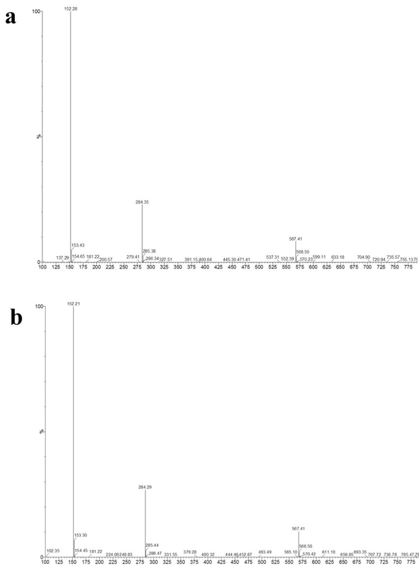
**Figure S3.** Mass spectra of D-G (a) and L-G (b) in  $\text{H}_2\text{O}$  at room temperature. No impurity peak was observed.
