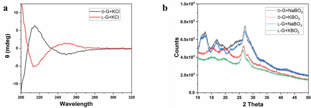
**Figure S14.** (a) CD spectrum of D-G (0.028% w/v) and L-G (0.014%) in KCl solution. (b) PXRD spectrum of D-G and L-G xerogels at concentration of 2.8% w/v in D<sub>2</sub>O.
