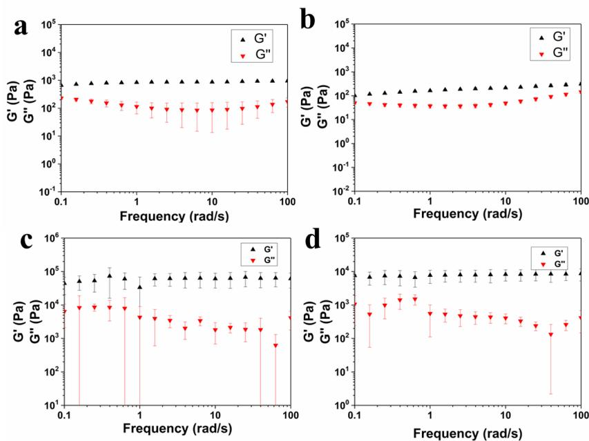
**Figure S17.** Frequency sweep test.  $G'$  at the angular frequency of 0.1 rad/s of D-G gel with KCl was 662.29 Pa (95% CI: 617.49 Pa, 707.08 Pa) (a), of L-G gel with KCl was 101.49 Pa (95% CI: 96.791 Pa, 106.18 Pa) (b), of D-G gel with NaBO<sub>3</sub> was 44287 Pa (95% CI: 11337 Pa, 77236 Pa) (c), of L-G gel with NaBO<sub>3</sub> was 7580.4 Pa (95% CI: 6370.7 Pa, 8430 Pa) (d); Data were analyzed by a Bonferroni multiple comparisons test after a significant ANOVA ( $P < 0.05$ ).
