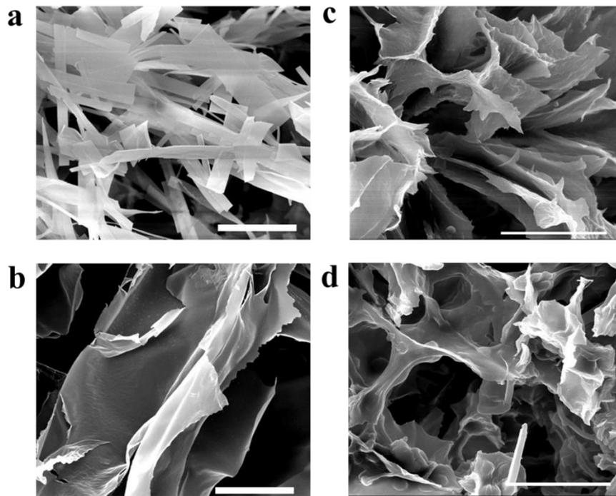
**Figure S16.** SEM images of xerogels. (a)(b) D-G+KCl (a) and L-G+KCl (b) gels at the concentration of 2.8% w/v (scale bar: 15  $\mu\text{m}$ ). (c)(d) D-G+NaBO<sub>3</sub>+PBS (c) and L-G+NaBO<sub>3</sub>+PBS (d) gels at the concentration of 2.8% w/v (scale bar: 20  $\mu\text{m}$ ).
