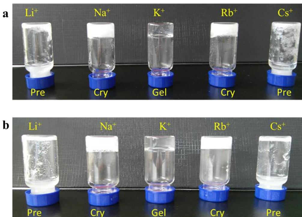
**Figure S1.** Inversion tests of 1.4% w/v D-G (a) and L-G (b) gels with different metal ions.
