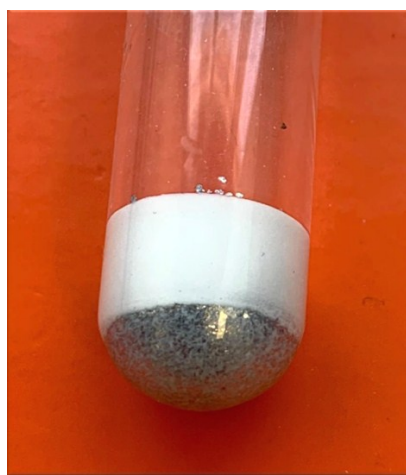
Figure S9 After conversion to conglomerate the denser zinc powder was separated from amino acid by centrifugation.
