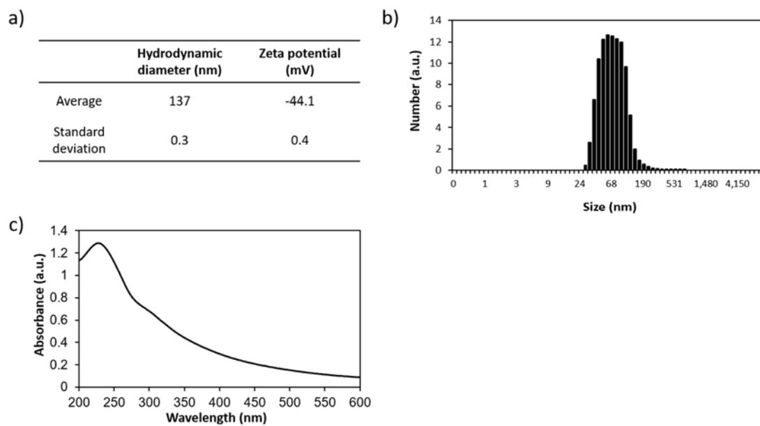
**Figure S1** Characterization of NGO. a) Results of DLS and zeta potential analysis. b) The size distribution of NGO. c) UV-vis spectrum of NGO.
