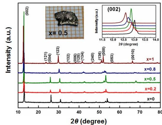
**Fig. 1** PXRD patterns of  $K_{0.8}Fe_{1.6}(S_{1-x}Se_x)_2$ , which can be indexed by  $I4/m$  space group. The left inset shows the optical photograph of the crystal sample with  $x=0.5$ , and the right inset shows the enlarged [002] diffraction peaks.
