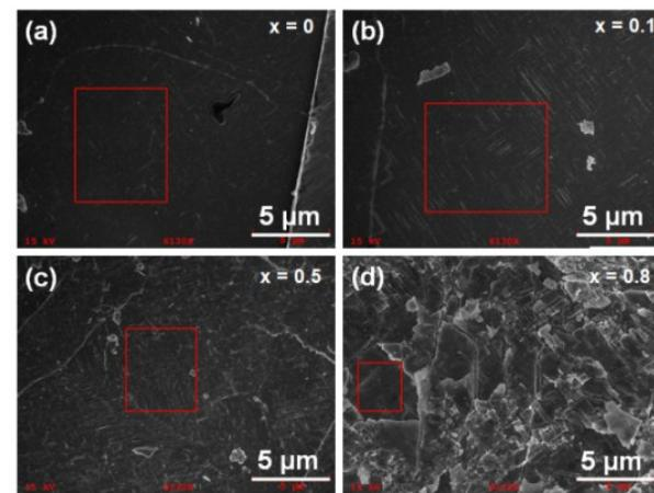
**Fig. S2** Morphology of  $FeS_{1-x}Se_x$  crystal sheets with  $x=$  (a) 0, (b) 0.1, (c) 0.5 and (d) 0.8. The red squares represent selected area for EDS measurements.
