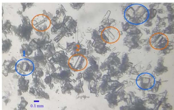
Fig. S1. An optical image of [\text{Zn}_2(\text{pypz})_2(\text{bdc})] crystals synthesized by using \text{Zn}(\text{NO}_3)_2 \cdot 6\text{H}_2\text{O} as metal salt and 5:1 DMF/ \text{H}_2\text{O} as solvent ( 1 and 2 are highlighted by blue and orange circles, respectively).
