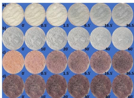
**Figure S15.** (a,b) Photochromism and color retention experiments of compound **1-Tm**; (c,d) Photochromism and color retention experiments of compound **2-Er**.
