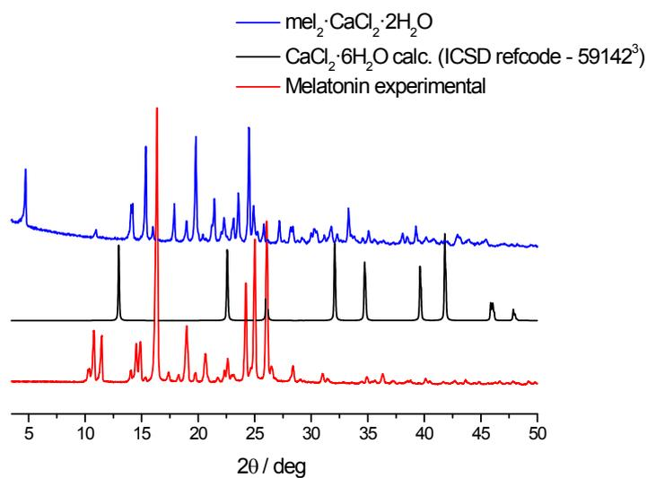
Figure ESI - 12. XRPD comparison between mel<sub>2</sub>·CaCl<sub>2</sub>·2H<sub>2</sub>O and starting materials. (Ref. 3: P. A. Agron and W. R. Busing, *Acta Crystallographica Section C Crystal Structure Communications*, 1986, **42**, 141-143.)
