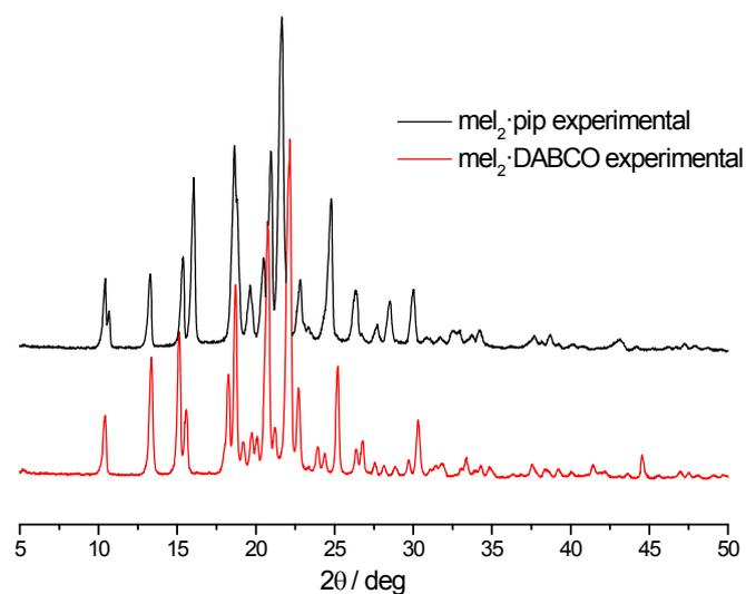
Figure ESI - 11. Comparison between the experimental XRPD pattern of mel<sub>2</sub>·pip and mel<sub>2</sub>·DABCO.
