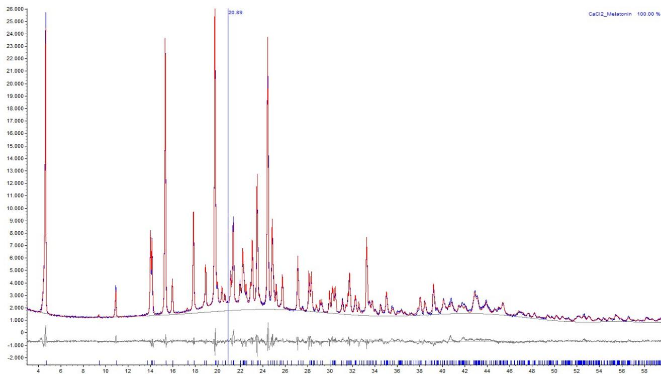
Figure ESI-13. Rietveld refinement of mel<sub>2</sub>-CaCl<sub>2</sub>·2H<sub>2</sub>O. R<sub>wp</sub>=4.83, R<sub>p</sub>=3.73, R<sub>exp</sub>=2.17,  $\chi^2$ =2.23.
