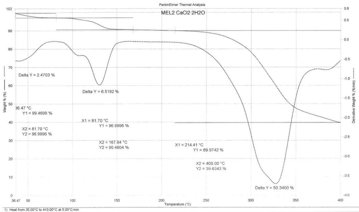
Figure ESI - 7. TGA trace of  $\text{mel}_2 \cdot \text{CaCl}_2 \cdot 2\text{H}_2\text{O}$ .
