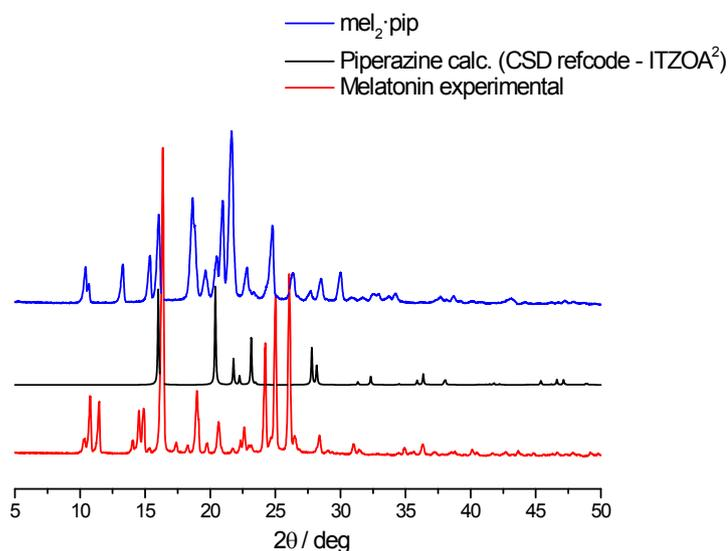
Figure ESI - 10. XRPD comparison between  $\text{mel}_2 \cdot \text{pip}$  and starting materials. (Ref. 2: A. Parkin, I. D. H. Oswald and S. Parsons, *Acta Crystallographica Section B Structural Science*, 2004, **60**, 219-227.)
