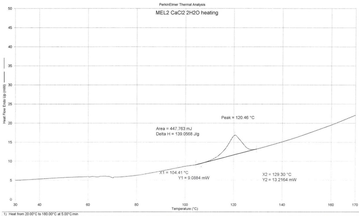
Figure ESI - 8. DSC trace of  $\text{mel}_2 \cdot \text{CaCl}_2 \cdot 2\text{H}_2\text{O}$ .
