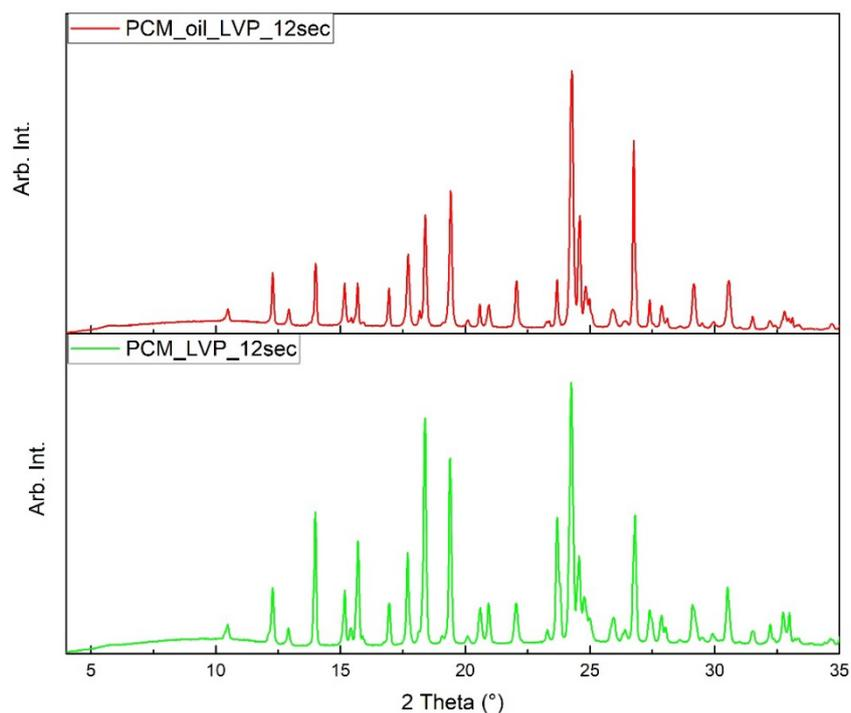
Figure S6. XRPD patterns obtained from samples produced by LVP experiment with (upper, red) and without (lower, green) inclusion of 500  $\mu$ l perfluorinated oil. Subtle difference in the patterns indicate differences in the relative amounts of PCM I and II in the sample mixtures.
