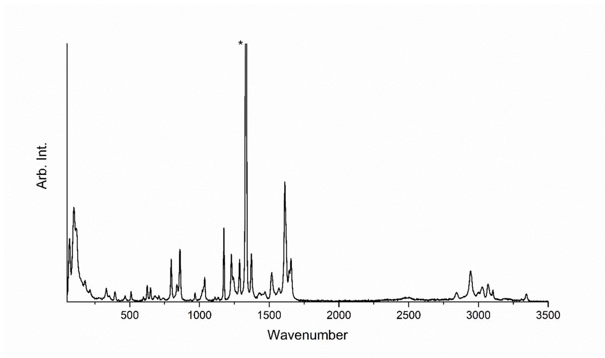
Figure S9. Raman spectrum obtained from MeOH solvate of PCM obtained from 0.05 g/g solvent mixture solution at 0.2 GPa in diamond anvil cell. Peak at approx. 1330 cm<sup>-1</sup>, marked with asterisk, attributed to diamond.
