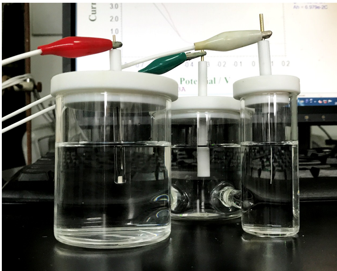
Fig. S5. The digital photograph of the typical three-electrode system.
