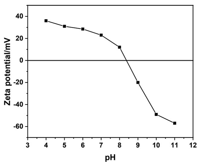
**Figure S8.** Zeta potential of natroalunite hexagonal nanoplate (S4') as a function of pH.
