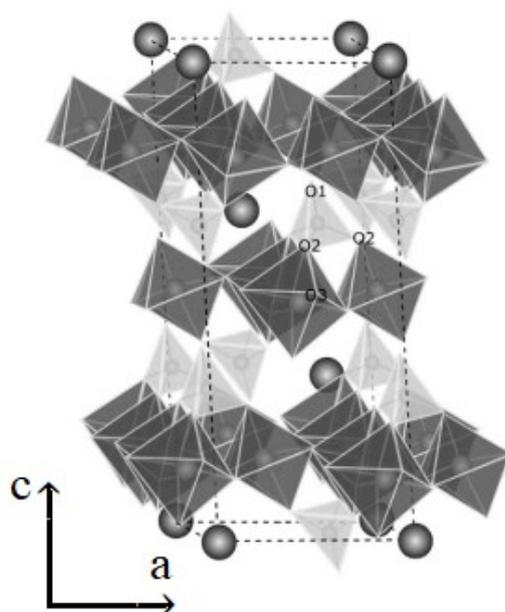
**Scheme S1.** Schema of the natroalunite structure.† The dashed lines show the unit cell. SO<sub>4</sub> groups are the light colored tetrahedra, Al–O<sub>2</sub>(OH)<sub>4</sub> octahedra are dark grey and the large spheres represent Na. The SO<sub>4</sub> group is triply coordinated with Al–O<sub>2</sub>(OH)<sub>4</sub> octahedra through the O<sub>2</sub> atom, whereas the O<sub>1</sub> (apical) atom is not coordinated. The O<sub>3</sub> atom is linked as OH group (H atoms are not shown).
