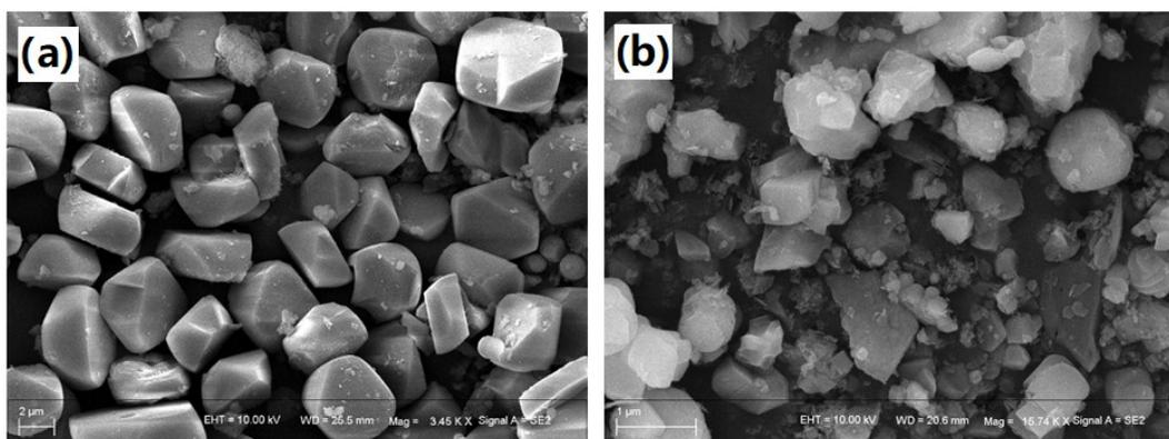
**Figure S2.** The FE-SEM images of as-prepared products without ionic liquid for 10 h (a: 130 °C, b:150 °C).
