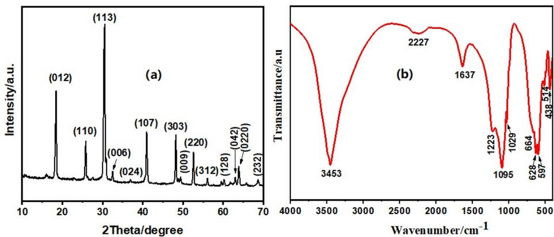
**Figure S1.** XRD pattern (a) and FTIR spectrum (b) of as-prepared product (S-4': 5 mmol of  $[C_{12}mim]Cl$  at 150 °C for 10 h).
