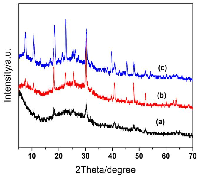
**Figure S5.** XRD spectra of the products obtained with different amount of AcNa at 130 °C for 2 h (a: 2.5, b: 5, c: 7.5 mmol).
