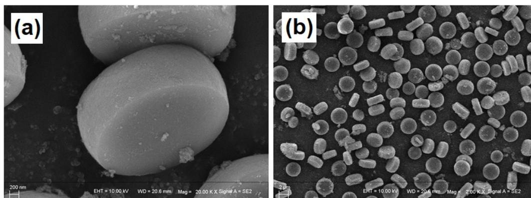
**Figure S9.** The FE-SEM images of as-prepared product with ionic liquid [Bmim] at
