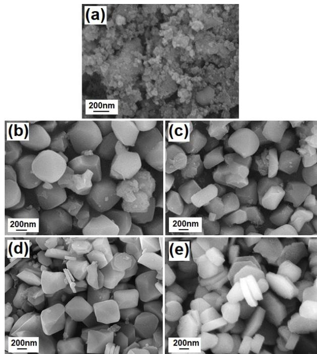
**Figure S4.** The FE-SEM images of the samples at 150 °C for (a) 1, (b) 2, (c) 3, (d) 5 and (e) 7 h, respectively.
