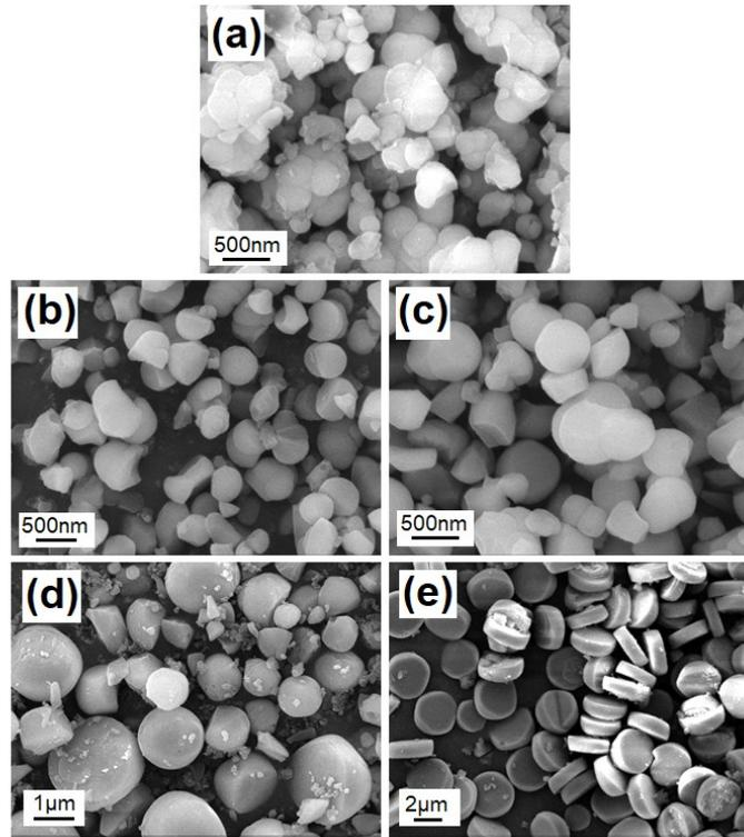
**Figure S3.** The FE-SEM images of the samples at 130 °C for (a) 1, (b) 2, (c) 3, (d) 5 and (e) 7 h, respectively.
