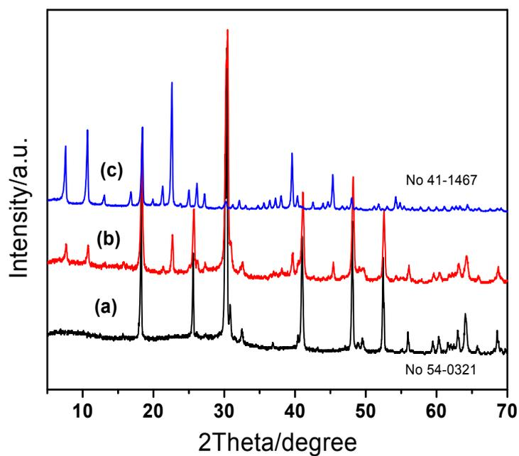
**Figure S6.** XRD spectra of the products obtained with different amount of AcNa at 130 °C for 10 h (a: 2.5, b: 5, c: 7.5 mmol).
