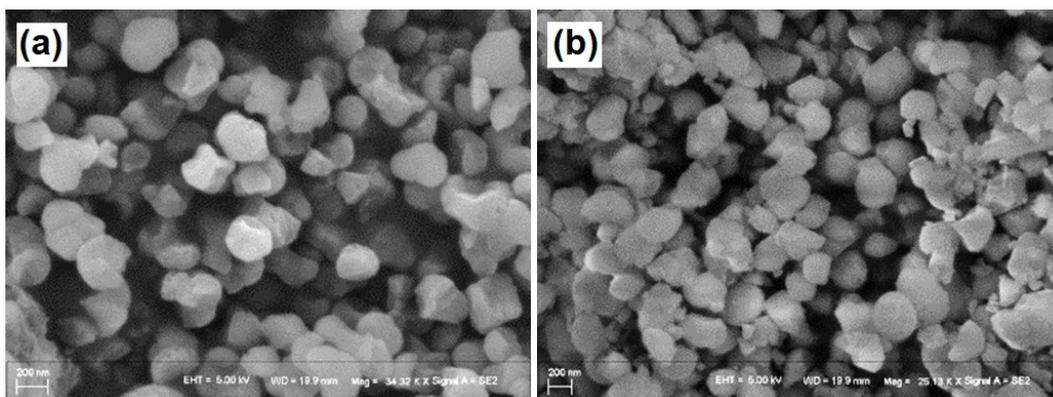
**Figure S7.** SEM images of the products obtained with different amount of AcNa at 130 °C for 10 h (a: 5, b: 7.5mmol).
