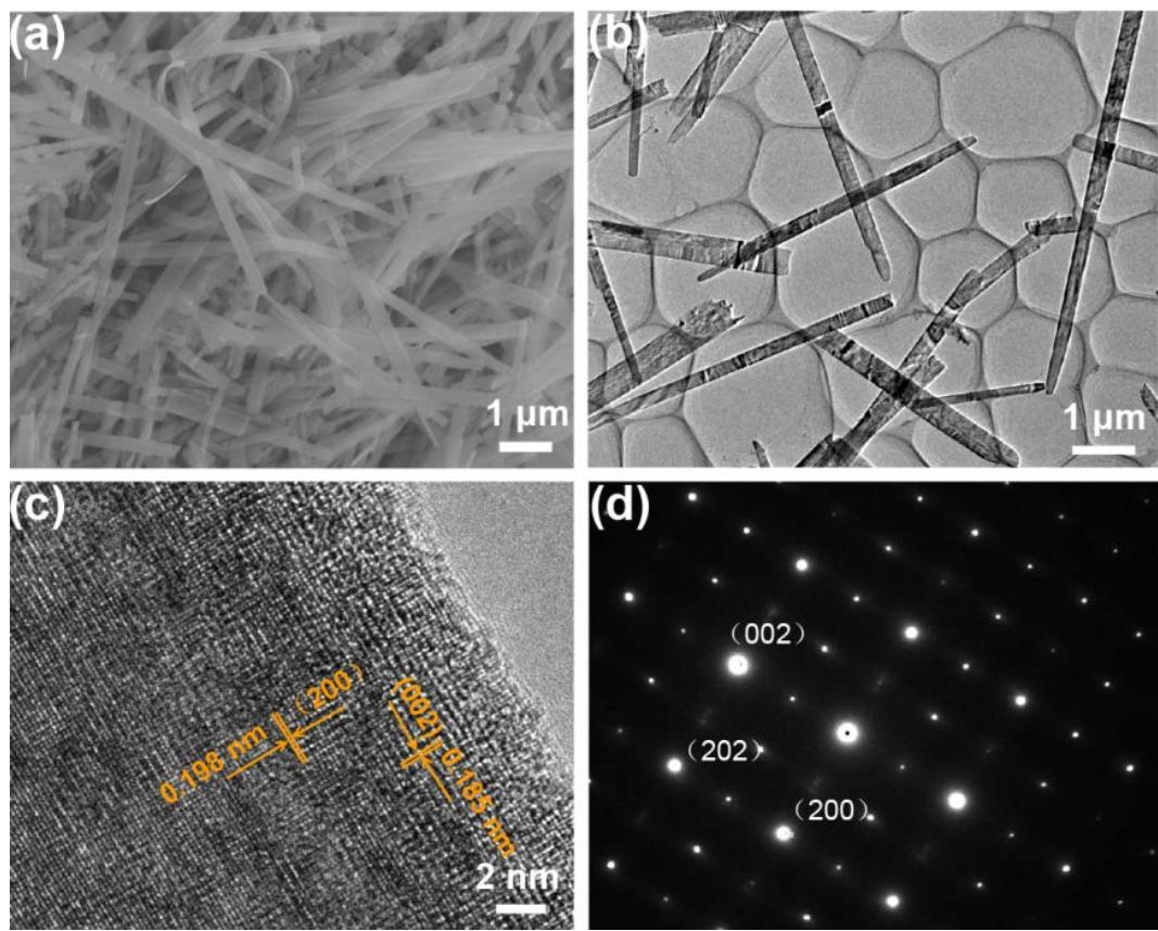
**Fig. S1†.** (a) The SEM image, (b) Typical TEM image and (c) HRTEM pattern, (d) SAED image of  $\text{MoO}_3$  NRs.
