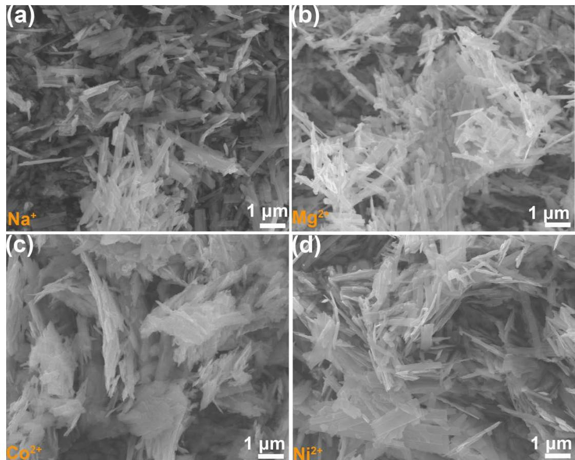
**Fig. S2†** The SEM images of samples obtained with different cations: (a)  $\text{NaNO}_3$ , (b)  $\text{Mg}(\text{NO}_3)_2 \cdot 6\text{H}_2\text{O}$ , (c)  $\text{Co}(\text{NO}_3)_2 \cdot 6\text{H}_2\text{O}$ , (d)  $\text{Ni}(\text{NO}_3)_2 \cdot 6\text{H}_2\text{O}$
