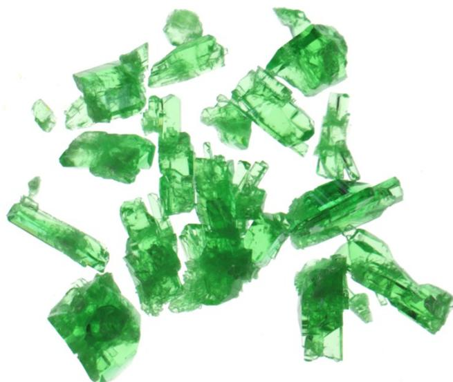
**Figure S3.** Photograph of Ni-BTC crystals under daylight.
