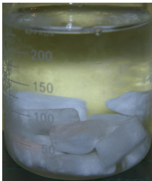
Fig. S9 Photo of samples mineralized in the CaCl 2 solution.
