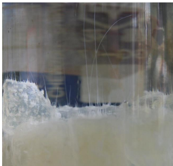
Fig. S11 Photo of the sample prepared using agar gel as template (mineralized in the \text{Na}_3\text{PO}_4 solution).
