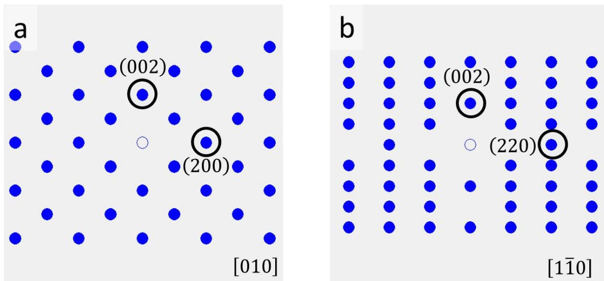
**Fig. S3** Simulated electron diffraction patterns of Anilite phase (1251523, Pearson's crystal data) along zone axes: (a)  $[010]$  and (b)  $[1\bar{1}0]$ .
