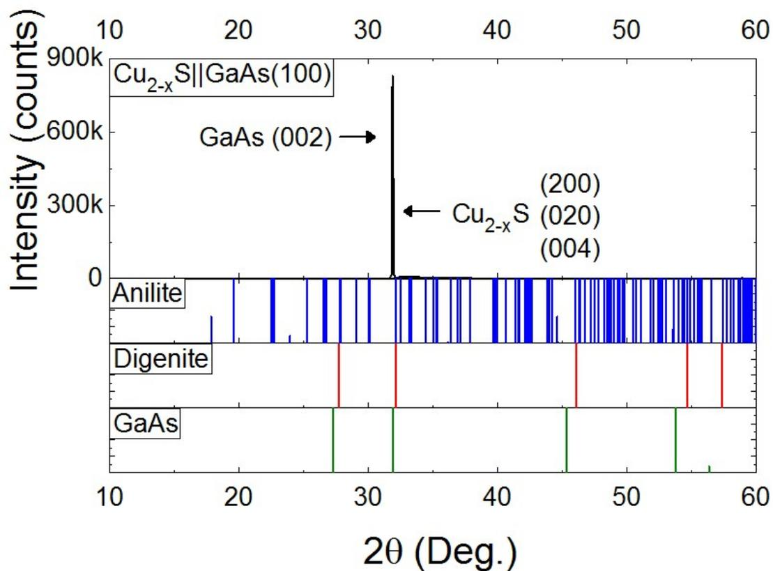
**Fig. S2** Wide  $2\theta$  range X-ray diffractogram of  $\text{Cu}_{2-x}\text{S}$  thin films deposited on GaAs(100) at temperature of  $70^\circ\text{C}$  for growth duration of 5 hr,  $\text{Cu}_{2-x}\text{S}$  – Anilite (1251523, Pearson’s crystal data),  $\text{Cu}_{2-x}\text{S}$  - Digenite (455552, Pearson’s crystal data) and GaAs – zinc blende (453930, Pearson’s crystal data). See Fig.3 in main text for a magnified and resolved view of the region  $2\theta \approx 32$  degrees.
