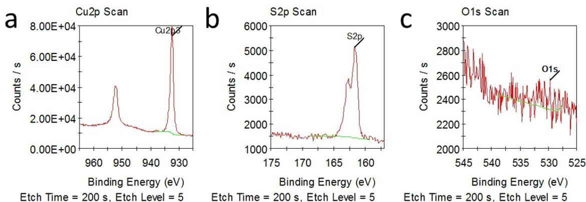
**Fig. S1** High-resolution XPS of etched  $\text{Cu}_{2-x}\text{S}$  thin films deposited on GaAs(100). Cu with 2p<sub>3/2</sub> photoelectron peaks indicate binding energies of 932.5 eV and 952.3 eV (b) S - 2p photoelectron peak show binding energies of 161.7 eV and 162.8 eV. (c) O - 1s photoelectron peak is indistinguishable.
