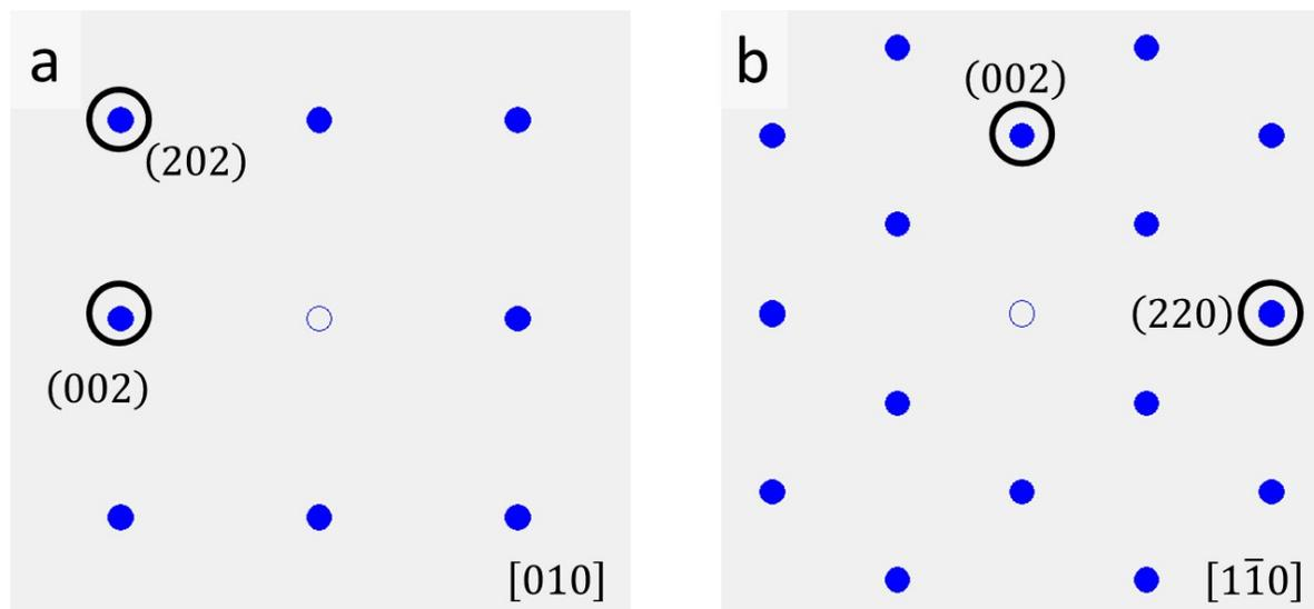
**Fig. S4** Simulated electron diffraction patterns of Digenite phase (455552, Pearson's crystal data) along zone axes: (a)  $[010]$  and (b)  $[1\bar{1}0]$ .
