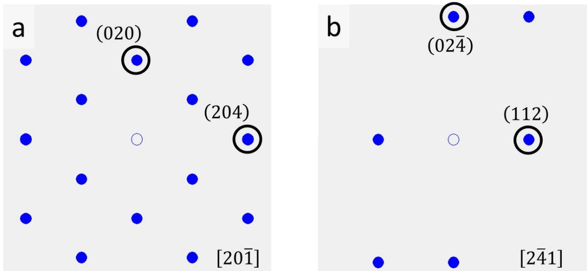
**Fig. S6** Simulated electron diffraction patterns of base-centered orthorhombic (BCO)  $\text{Cu}_{2-x}\text{S}$  phase with lattice parameters  $a \approx b = 5.6 \text{ \AA}$  and  $c = 11.2 \text{ \AA}$  viewed along zone axes  $[20\bar{1}]$  and  $[2\bar{4}1]$ .
