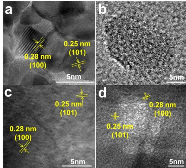
Fig. S.2 HRTEM images of (a) ZnO-0, (b) ZnO-1, (c) ZnO-2 and (d) ZnO-3.
