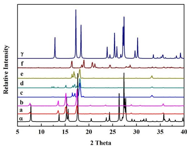
Fig. S9 X-ray powder diffraction patterns of obtained PZA crystals with hydrochlorothiazide (a: without templates; b: with amorphous templates; c: with physical mixture of crystalline templates: amorphous template = 1:4; d: with physical mixture of crystalline templates: amorphous template = 3:2; e: with crystalline templates; f: crystalline hydrochlorothiazide.), along with the simulated PXRD pattern of  $\alpha$  form and  $\gamma$  form of PZA.
