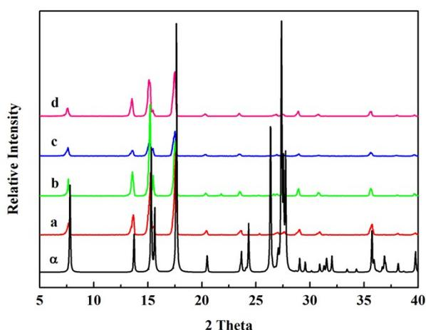
Fig. S7 X-ray powder diffraction patterns of obtained PZA crystals with a: soluble crystalline hydrochlorothiazide; b: with soluble amorphous hydrochlorothiazide; c: with soluble crystalline sulfathiazide; d: with soluble amorphous sulfathiazide, along with the simulated PXRD pattern of  $\alpha$  form of PZA.
