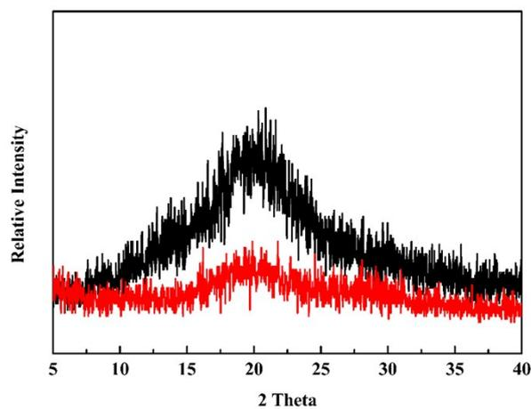
Fig. S8 X-ray powder diffraction patterns of amorphous hydrochlorothiazide (black line) and amorphous sulfathiazole (red line).
