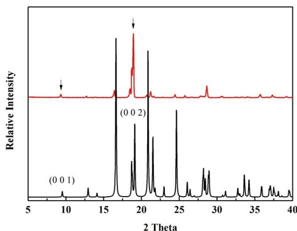
Figure S1. X-ray powder diffraction patterns of hydrochlorothiazide (red line), along with the simulated PXRD pattern (black line).
