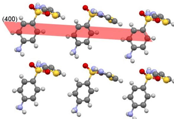
Figure S6. View of the (4 0 0) face of sulfathiazole (view along b axis).
