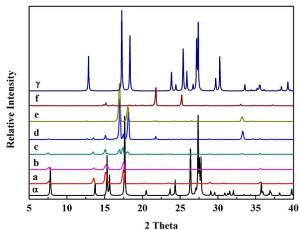
Fig. S10 X-ray powder diffraction patterns of obtained PZA crystals with sulfathiazole (a: without templates; b: with amorphous templates; c: with physical mixture of crystalline templates: amorphous template = 1:4; d: with physical mixture of crystalline templates: amorphous template = 3:2; e: with crystalline templates; f: crystalline sulfathiazole.), along with the simulated PXRD pattern of  $\alpha$  form and  $\gamma$  form of PZA.
