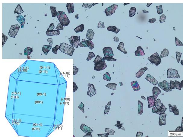
Figure S2. Microscope images of hydrochlorothiazide, imbedded image is BFDH morphology of hydrochlorothiazide calculated by Mercury.
