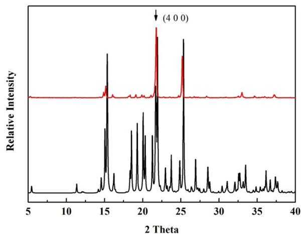
Figure S4. X-ray powder diffraction patterns of sulfathiazole (red line), along with the simulated PXRD pattern (black line).
