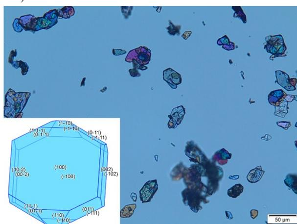
Figure S5. Microscope images of sulfathiazole, imbedded image is BFDH morphology of sulfathiazole calculated by Mercury.
