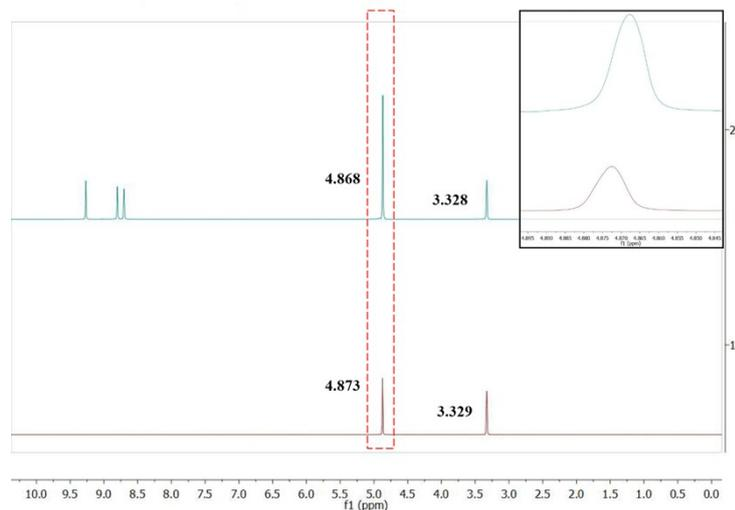
Fig. S12  $^1\text{H}$  NMR spectra of methanol- $\text{d}_4$  and pyrazinamide-methanol- $\text{d}_4$  solution. (The signals in red dashed box are from hydroxyl hydrogen.)
