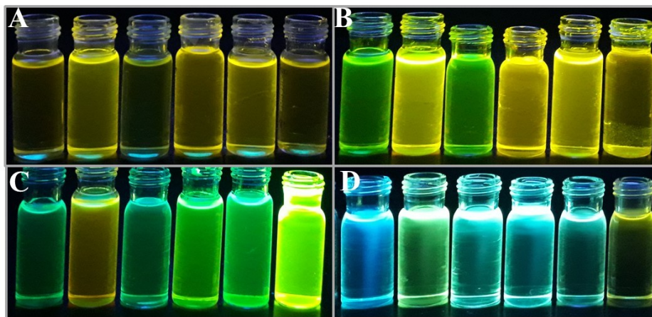
Figure S20. Fluorescence photographs of (A) L 1 (B) L 2 (C) L 3 and (D) L 4 in various organic solvents ranging from low polarity to high polarity (10 \mu M) under UV lamp (365 nm). Toluene; chloroform; tetrahydrofuran; dimethyl sulfoxide; acetonitrile; methanol.
