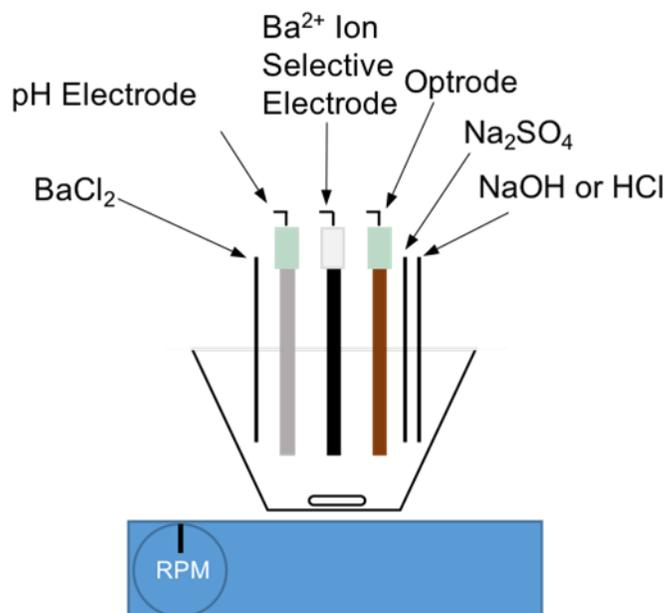
**Fig. S5.** Schematic of the titration setup with Barium ISE, pH electrode and optrode, and nozzles for addition of all chemical species. The setup was modified as required for the different experiments by removing or adding extra accessories and plugging the ports.
