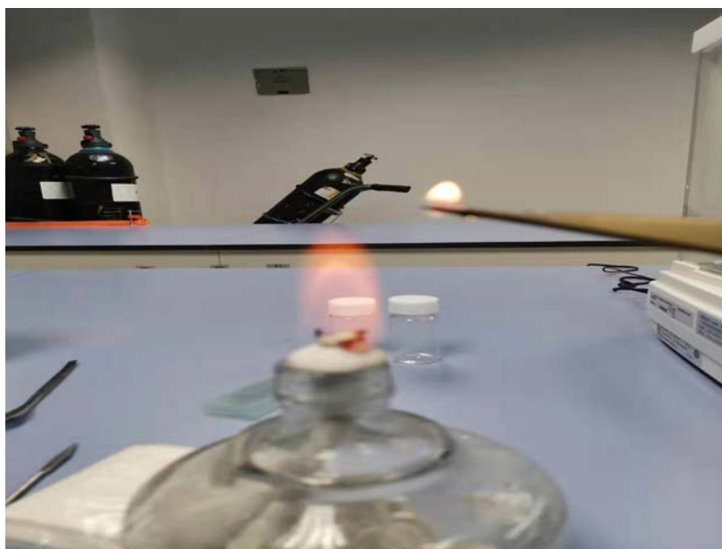
Figure S7. Flammability of commercial PP separator.
