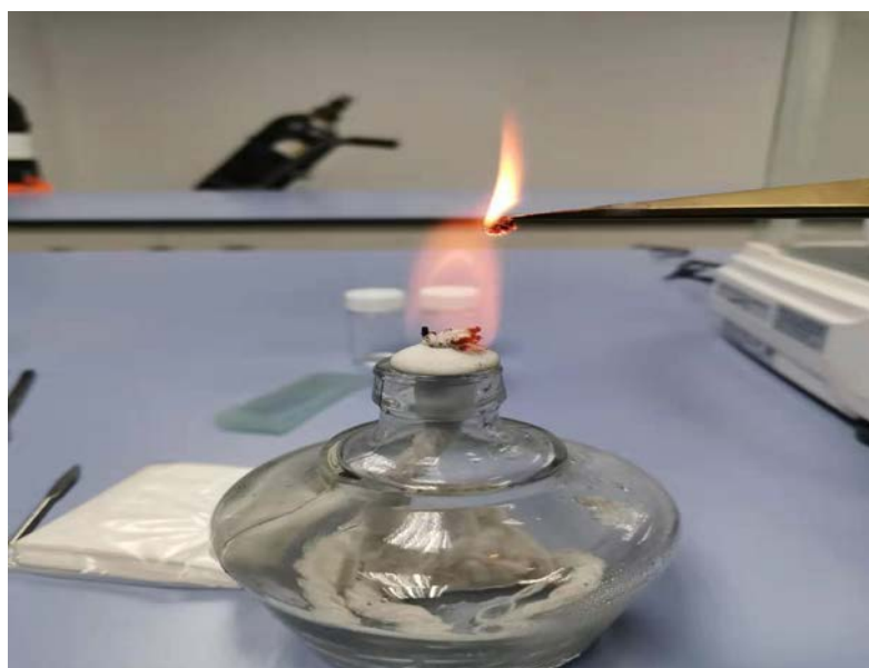
Figure S9. Flammability of electrospun PAEK-Al 2 O 3 composite separator.
