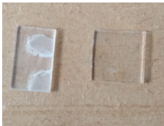
Figure S6: Comparison of glass slide covered using the RTD approach after 5 h at 150°C (left) with uncoated glass slide (right). The white areas of unreacted starting material are visible, while the rest of the glass slide is slightly opaque in comparison with the uncoated glass slide, implying coating of the surface.
