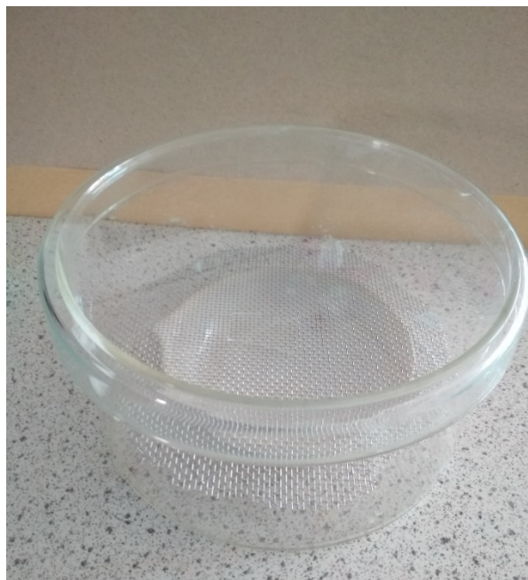
Figure S7: Experimental set-up used for the vapour-assisted conversion.
