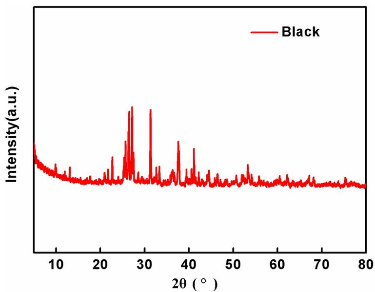
**Figure S8.** XRD patterns of the nanotubes after heating treatment(330°C).
