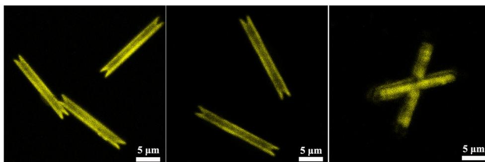
**Figure S14.** Confocal microscopy images of the nanotubes with the same control parameters. (a) fresh preparation; (b) stored in hexane at 4 °C for 10 months; (c)
