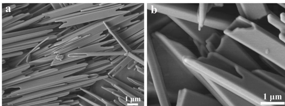
**Figure S9.** Representative hollow SEM images of the as-prepared CsPbI<sub>3</sub> nanotubes.
