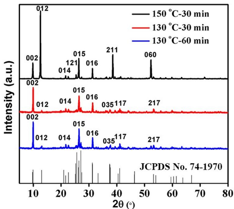
**Figure S6.** XRD patterns of the nanotubes at different reaction temperature and different reaction time.
