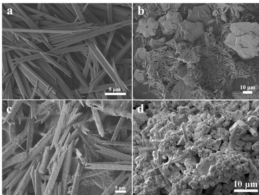
**Figure S11.** Representative morphologies of the CsPbI<sub>3</sub> (a, b, c) and PbI<sub>2</sub> (d) with different synthetic conditions (see Table S1).
