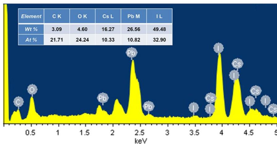
**Figure S2.** Energy dispersive X-ray spectroscopy analysis of the CsPbI<sub>3</sub> nanotubes.
