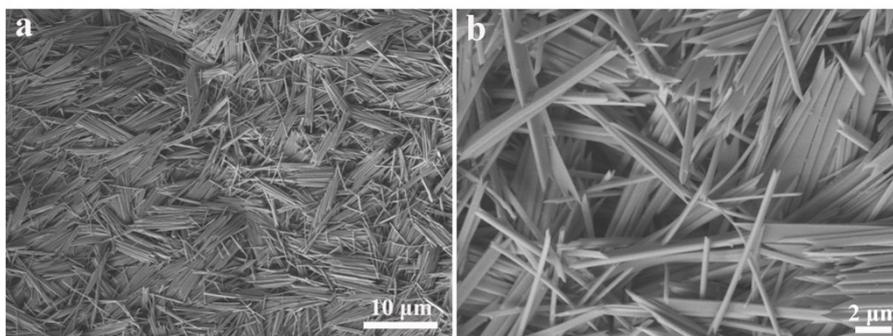
**Figure S5.** Representative SEM images of the as-prepared CsPbI<sub>3</sub> nanotubes synthesized at 110°C under different magnifications.
