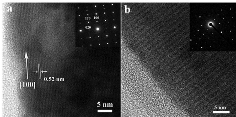
**Figure S1.** HR-TEM image and corresponding SAED of CsPbI<sub>3</sub> nanotubes in different regions.
