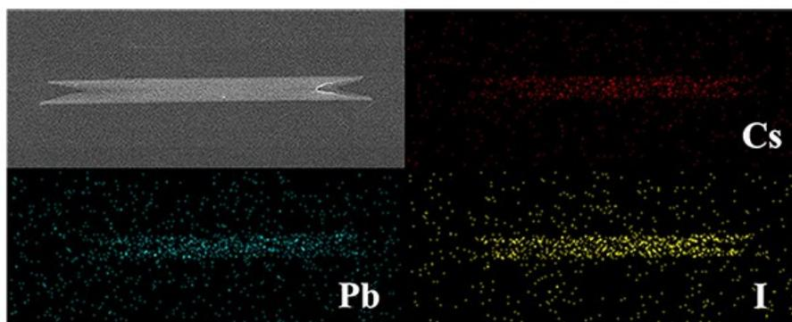
**Figure S3.** EDS mapping of the nanotubes, showing the uniform elemental distribution of Cs, Pb, I.
