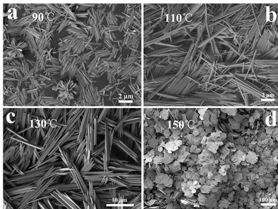
**Figure S4.** Representative SEM images of the as-prepared CsPbI<sub>3</sub> nanotubes synthesized with different reaction temperature with a fixed reaction time of 30 min.
