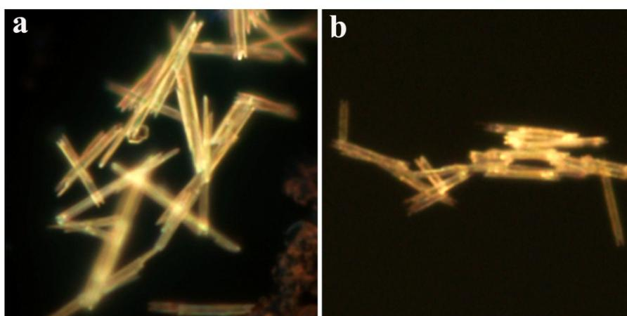
**Figure S13.** Microphotographs of CsPbI<sub>3</sub> nanotubes under excitation at 365 nm.
