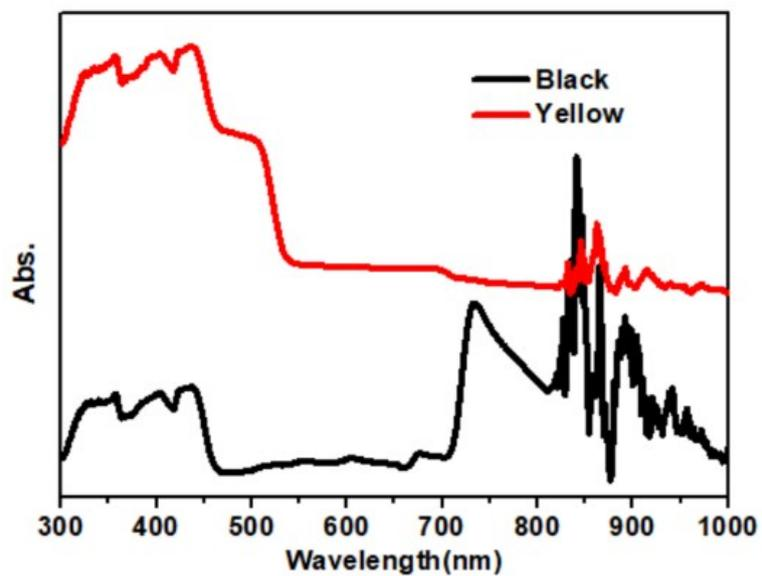
**Figure S7.** UV-vis absorption spectrum of the nanotubes before and after heating (330°C) treatment in a vacuum.
