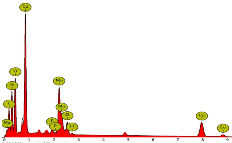
Figure S5 The EDS spectrum of **Cu-POM**.
