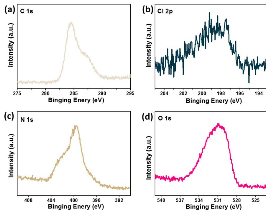
Figure S4 XPS spectra of **Cu-POM**: (a) C 1s, (b) Cl 2p, (c) N 1s, (d) O 1s, respectively.
