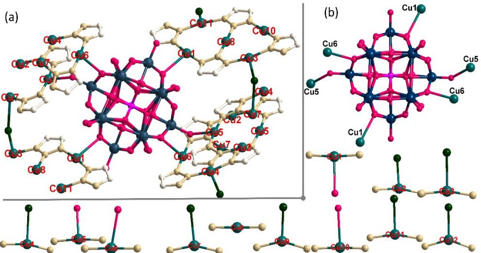
Figure S1 Ball/stick view of the crystallographic unit and the coordination patterns of PMo<sub>12</sub> and Cu ions of **Cu-POM**. All of the hydrogen atoms were omitted for clarity.
