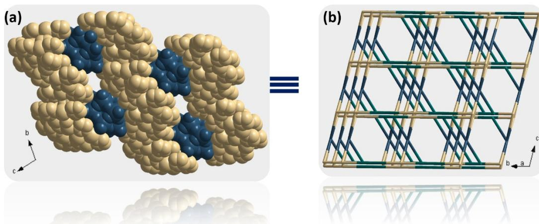
Figure S3 Combined stacked (a) and topologic (b) representation of 3D POM-based hybrid frameworks of **Cu-POM** with opening hole constructed by PMo<sub>12</sub> cluster as pillars and the double chains.
