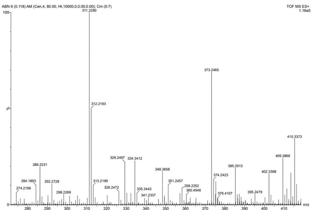
**Fig. S3.** HRMS spectrum of the receptor **N1**.
