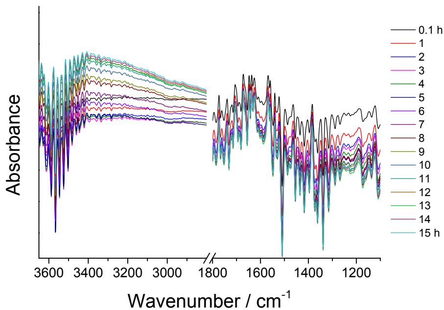
**Figure S14.** TG-IR spectra of LiTf<sub>2</sub>N:NMA (1:4 mol ratio, 12.2700 mg) at 27 °C at N<sub>2</sub> atmosphere in alumina pan for 15 h measured by the couple of Mettler Toledo TGA/DSC3+ with Thermo Scientific Nicolet iS50 FT-IR.
