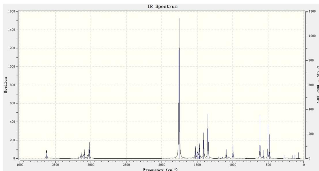
**Figure S9. Simulated IR spectra of NMA via Gaussian calculation by B3LYP/6-31++g(d,p) method.**
