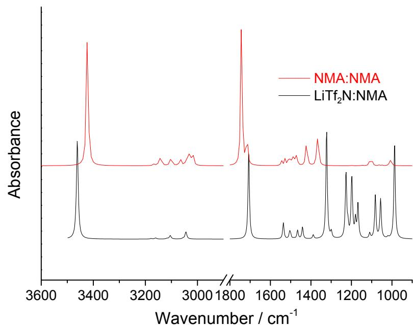
**Figure S13.** Comparison of the simulated IR spectra for NMA:NMA and LiTf<sub>2</sub>N:NMA via Gaussian calculation by B3LYP/6-31++g(d,p) method.
