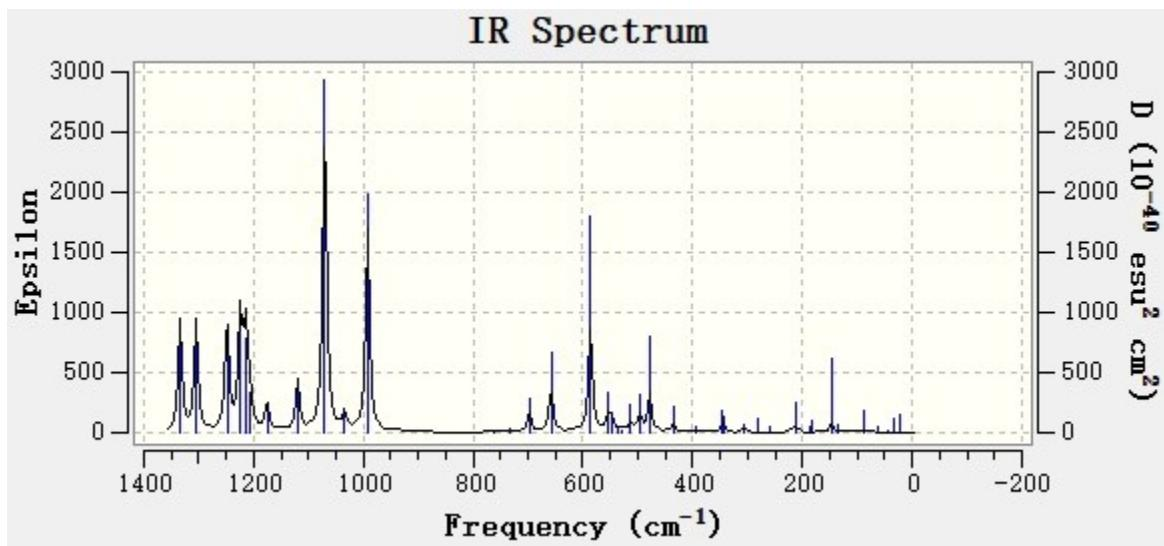
**Figure S10.** Simulated IR spectra of  $\text{LiTf}_2\text{N}$  via Gaussian calculation by B3LYP/6-31++g(d,p) method.
