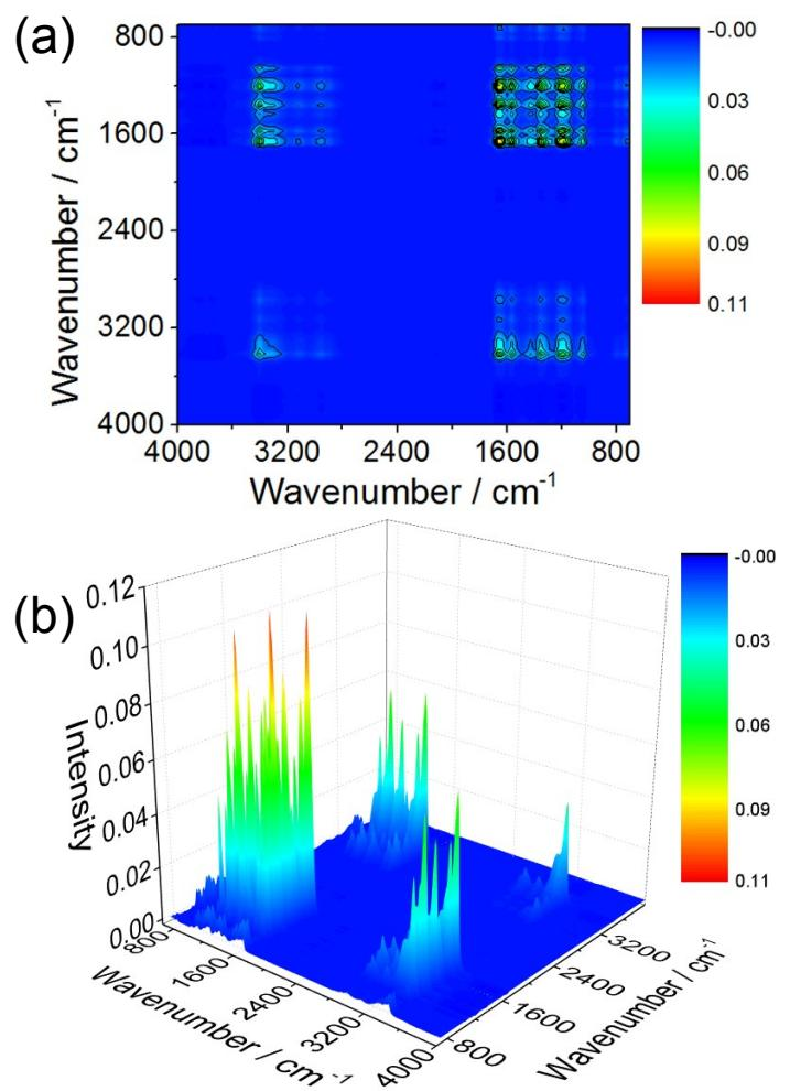
**Figure S4. Synchronous G-2DCOS spectra for DESs LiTf<sub>2</sub>N:NMA perturbated with time in the planar (a) and stereoscopic (b) mode.**
