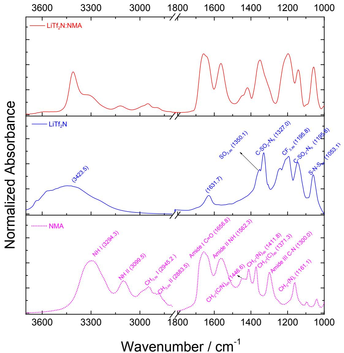
**Figure S6.** IR assignment for the reactants of DES: NMA and LiTf<sub>2</sub>N.
