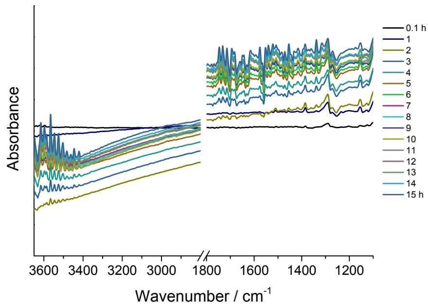
**Figure S16.** TG-IR spectra of pure water (19.3900 mg) at 27 °C at N<sub>2</sub> atmosphere in alumina pan for 15 h measured by the couple of Mettler Toledo TGA/DSC3+ with Thermo Scientific Nicolet iS50 FT-IR.
