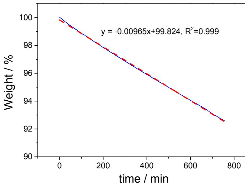
**Figure S3.** Weight change of DESs LiTf<sub>2</sub>N:NMA (5.00600 mg) as a function of time at 20 °C in TGA. The blue solid line is the measured data. The red dash line is the fitted curve.
