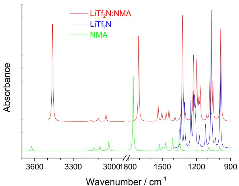
**Figure S12.** Comparison of the simulated IR spectra for NMA, LiTf<sub>2</sub>N and LiTf<sub>2</sub>N:NMA via Gaussian calculation by B3LYP/6-31++g(d,p) method.
