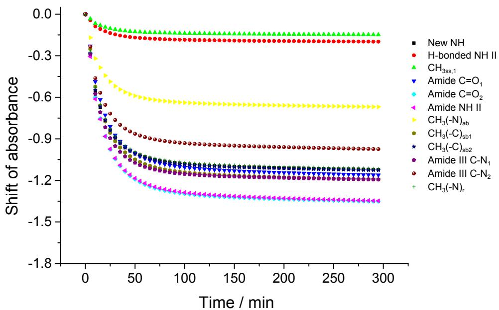
**Figure S1. Shift of intensity for difference IR peak absorbance of LiTf<sub>2</sub>N:NMA as a function of time.**
