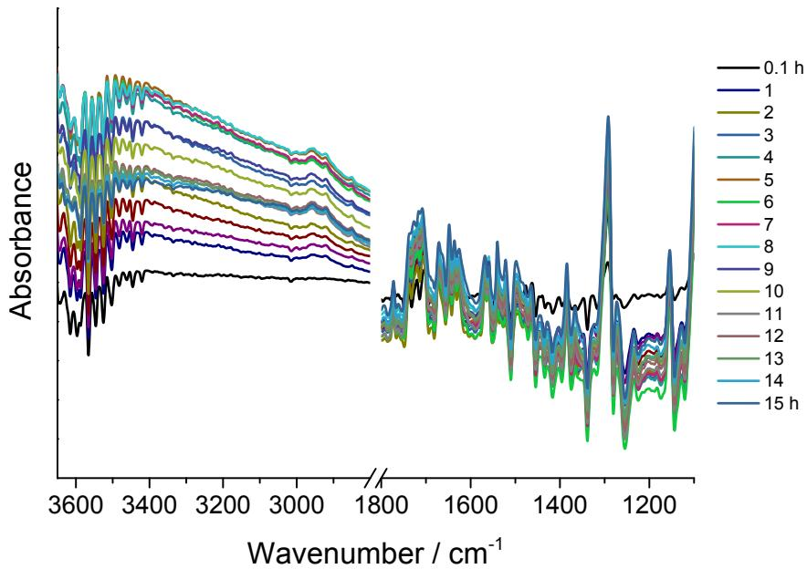
**Figure S15.** TG-IR spectra of pure NMA (15.4670 mg) at 27 °C at N<sub>2</sub> atmosphere in alumina pan for 15 h measured by the couple of Mettler Toledo TGA/DSC3+ with Thermo Scientific Nicolet iS50 FT-IR.
