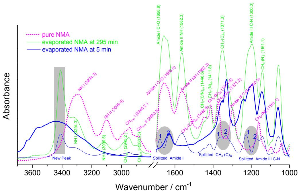
**Figure S7.** IR assignment for pure NMA and the evaporated NMA from DES LiTf<sub>2</sub>N:NMA (1:4).
