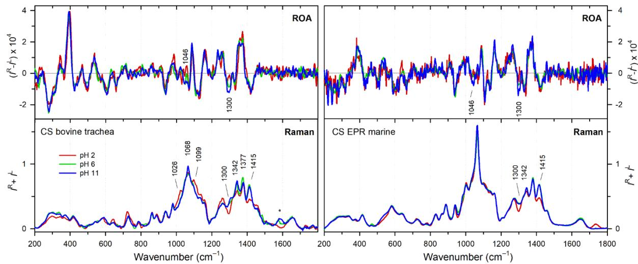
**Fig. S3** Raman and ROA spectra of CS from bovine trachea (left) and CS EPR marine (right) at neutral (pH 6, green), basic (pH 11, blue), and acidic (pH 2, red) environment. The major changes in spectra are labelled. The band at  $1590 \text{ cm}^{-1}$  corresponding to sample's impurities is marked by asterisk.
