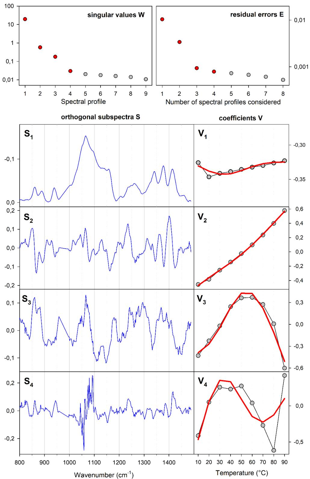
**Fig. S6** The factor analysis of Raman spectra temperature dependence of CS bovine trachea. Result of the one-step transition fit is shown by red lines.
