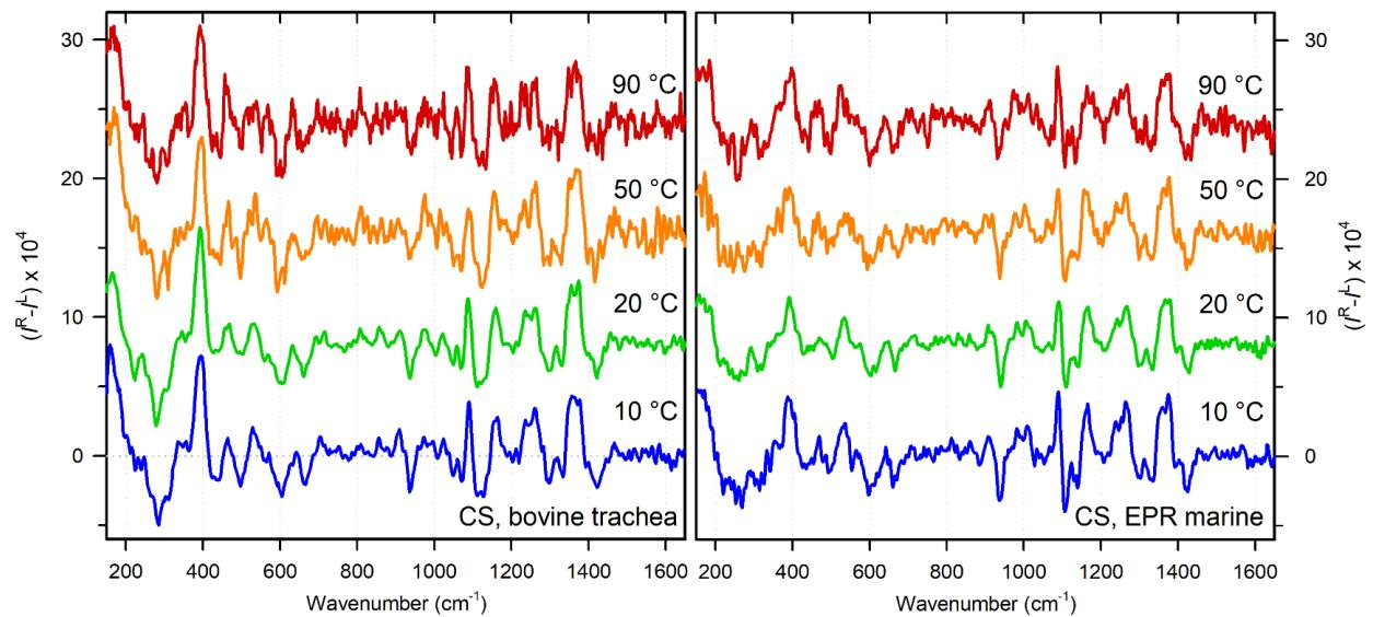
**Fig. S7** ROA spectra of CS from bovine trachea (left) and CS EPR marine (right) at various temperatures. The spectra belong to the Raman spectra in Fig. S4 and Fig. 8 measured at each corresponding temperature. The same factor was used for normalization of both Raman and ROA spectra.
