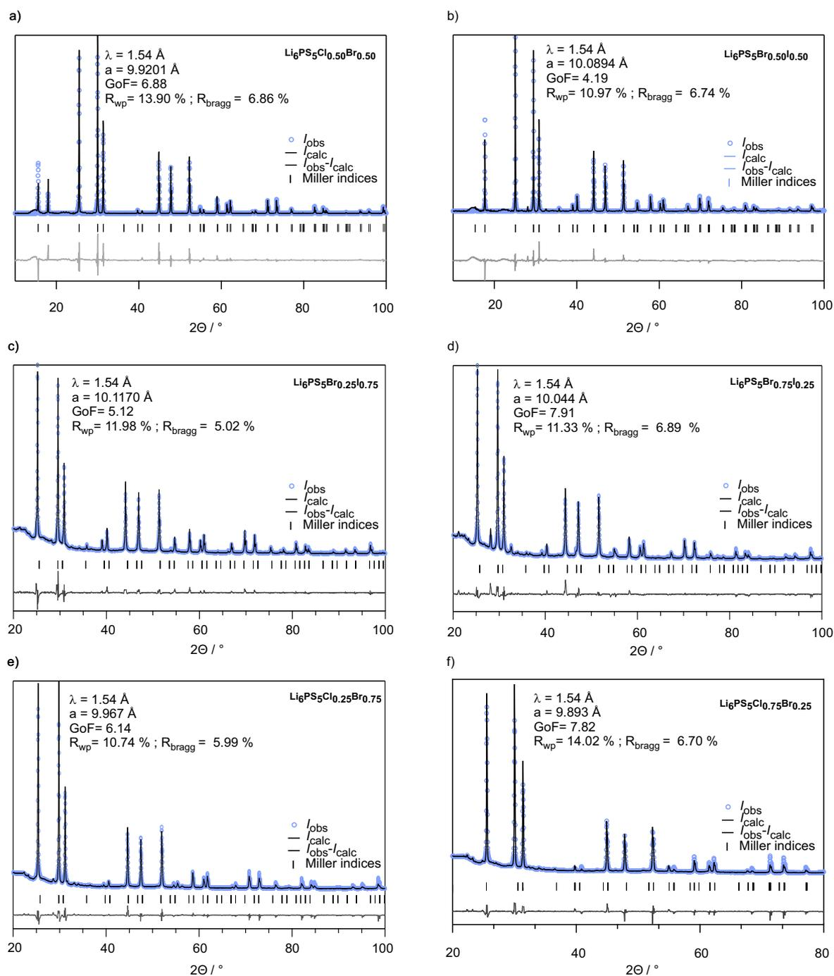
**Fig. S2** X-ray powder diffraction patterns and crystallographic data from Rietveld analyses of the Li-argyrodites indicated. As in Fig. S1, GoF means goodness of fit (GoF), the weighted  $R$ -profile ( $R_{\text{wp}}$ ) and the  $R$ -Bragg ( $R_{\text{bragg}}$ ) values are also shown. The differential plot as well as the hkl indices are included, too. The hump at approximately  $25^\circ$  is due to the mercatpo foil, which was used for the measurement
