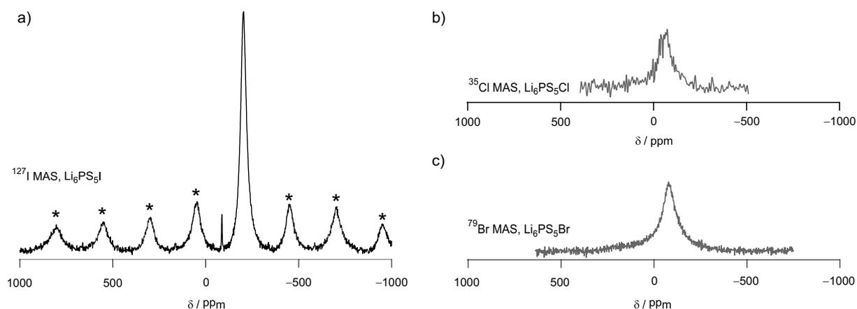
**Fig. S3**  $^{35}\text{Cl}$ ,  $^{79}\text{Br}$  and  $^{127}\text{I}$  MAS NMR spectra. Asterisks, see the NMR spectrum of  $\text{Li}_6\text{PS}_5\text{I}$ , denote spinning sidebands. The narrow line at  $-86.4\ \text{ppm}$  shows a negligible impurity phase.
