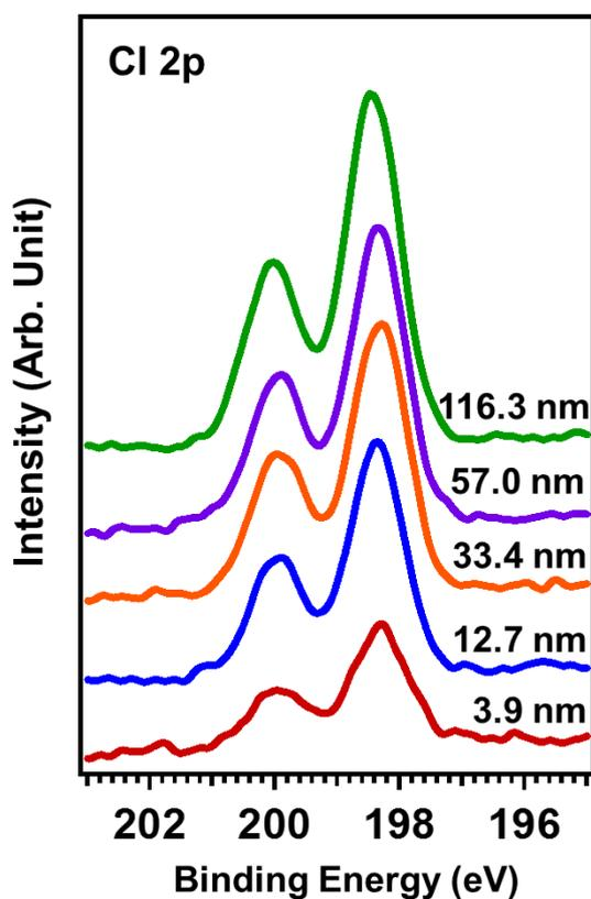
Figure S1. Cl 2p XPs spectra of perovskite films.
