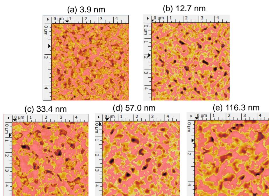
**Figure S4** AFM images used to calculate grain sizes (size: 5  $\mu\text{m}$   $\times$  5  $\mu\text{m}$ ) for (a) 3.9, (b) 12.7, (c) 33.4, (d) 57.0, and (e) 116.3 nm thick  $\text{CH}_3\text{NH}_3\text{PbI}_{3-x}\text{Cl}_x$  films.
