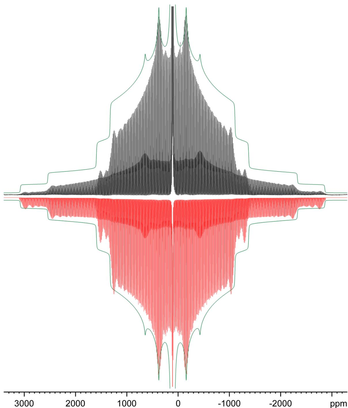
**Fig. S2** Experimental  $^{27}\text{Al}$  MAS NMR spectrum of  $\text{KAlH}_4$  measured at  $\nu_{\text{MAS}} = 1.4$  kHz (black) and its simulation (red) with the parameters  $\delta_{\text{iso}} = 107.6$  ppm,  $C_Q = 1.29$  MHz and  $\eta = 0.64$ . To ease the comparison, the simulated MAS NMR spectrum has been inverted. The green lines depict the lineshape one would obtain for a non-spinning sample.
