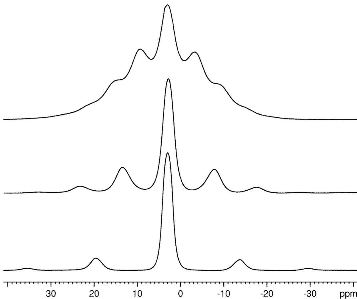
**Fig. S5** <sup>1</sup>H MAS NMR spectra of KAlH<sub>4</sub> recorded at different spinning frequencies  $\nu_{\text{MAS}}$ : 3 kHz (top), 5 kHz (middle), and 8 kHz (bottom). The experimental conditions are as follows: 500 MHz resonance frequency, 10 s repetition delay, and 3.0  $\mu\text{s}$   $\pi/4$  pulses. At  $\nu_{\text{MAS}} = 8$  kHz, the full width at half height of the line at 2.95 ppm amounts to about 1.3 kHz. The spectra give no indication of the presence of by-products.
