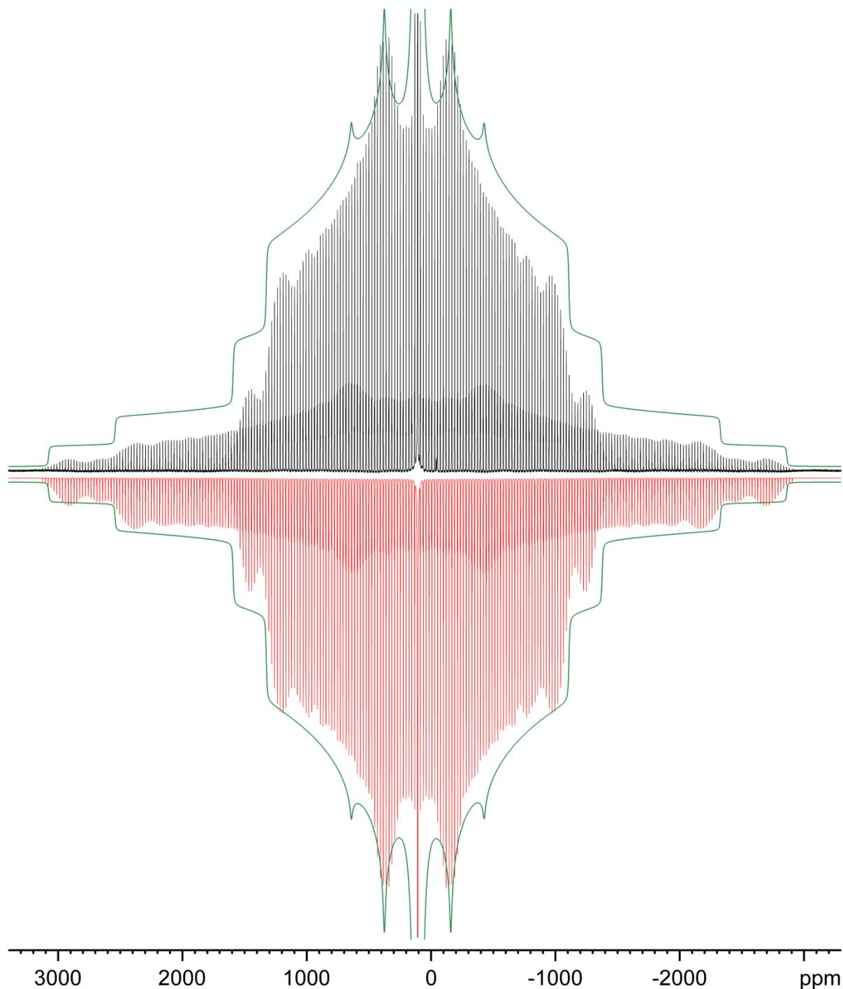
**Fig. S3** Experimental  $^{27}\text{Al}$  MAS NMR spectrum of  $\text{KAlH}_4$  measured at  $\nu_{\text{MAS}} = 3.0$  kHz (black) and its simulation (red) with the parameters  $\delta_{\text{iso}} = 107.6$  ppm,  $C_Q = 1.29$  MHz and  $\eta = 0.64$ . To ease the comparison, the simulated MAS NMR spectrum has been inverted. Again, the green lines depict the lineshape one would obtain for a non-spinning sample.
