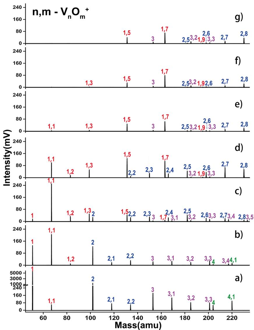
**Fig. S1** Full mass spectra of small  $V_n^+$  ( $n=1-4$ ) clusters produced via a 1.0 cm nozzle at the absence **(a)** and presence **(b-g)** of oxygen introduced into the reaction tube. The amount of oxygen (0.1 MPa 3% $O_2$ /He) is controlled by the on-time width of a pulsed valve: 210, 220, 230, 240, 250, 270  $\mu$ s, respectively.
