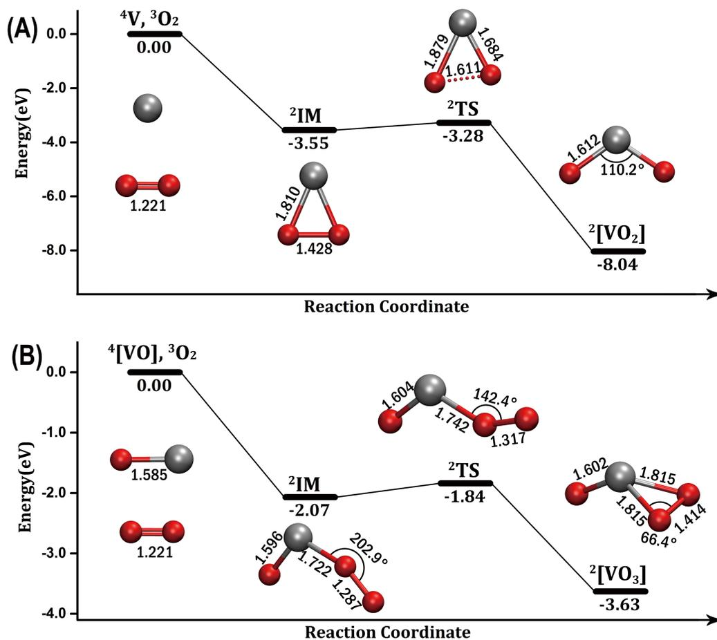
**Fig. S5** The calculated Reaction energy diagrams at BP86/def2TZVP level of theory. (A)  $V + O_2 \rightarrow VO_2$ , (B)  $VO + O_2 \rightarrow VO_3$ . The energy values are relative to the entrance channel, denoted as zero-point vibration corrected energies, and given in eV. Spin multiplicity is marked as pre-superscript.
