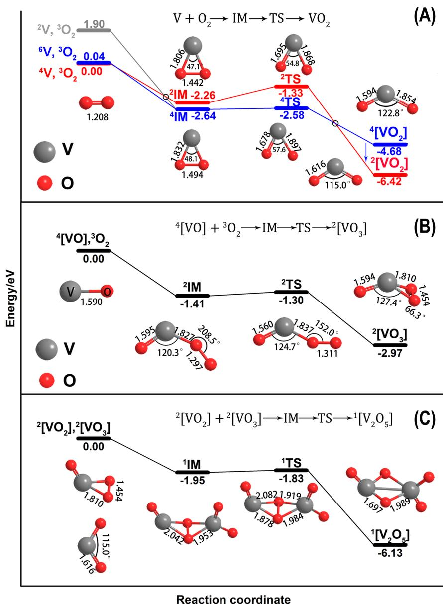
**Fig. S4.** Reaction energy diagrams of **(A)**  $V + O_2 \rightarrow VO_2$ , **(B)**  $VO + O_2 \rightarrow VO_3$ , and **(C)**  $VO_3 + VO_2 \rightarrow V_2O_5$ , calculated at B3LYP/TZVP level with DFT-D3 dispersion correction. The energy values are relative to the entrance channel, denoted as zero-point vibration corrected energies, and given in eV. Spin multiplicity is marked as pre-superscript. Hollow circle denotes a possible spin inversion point for reaction paths.
