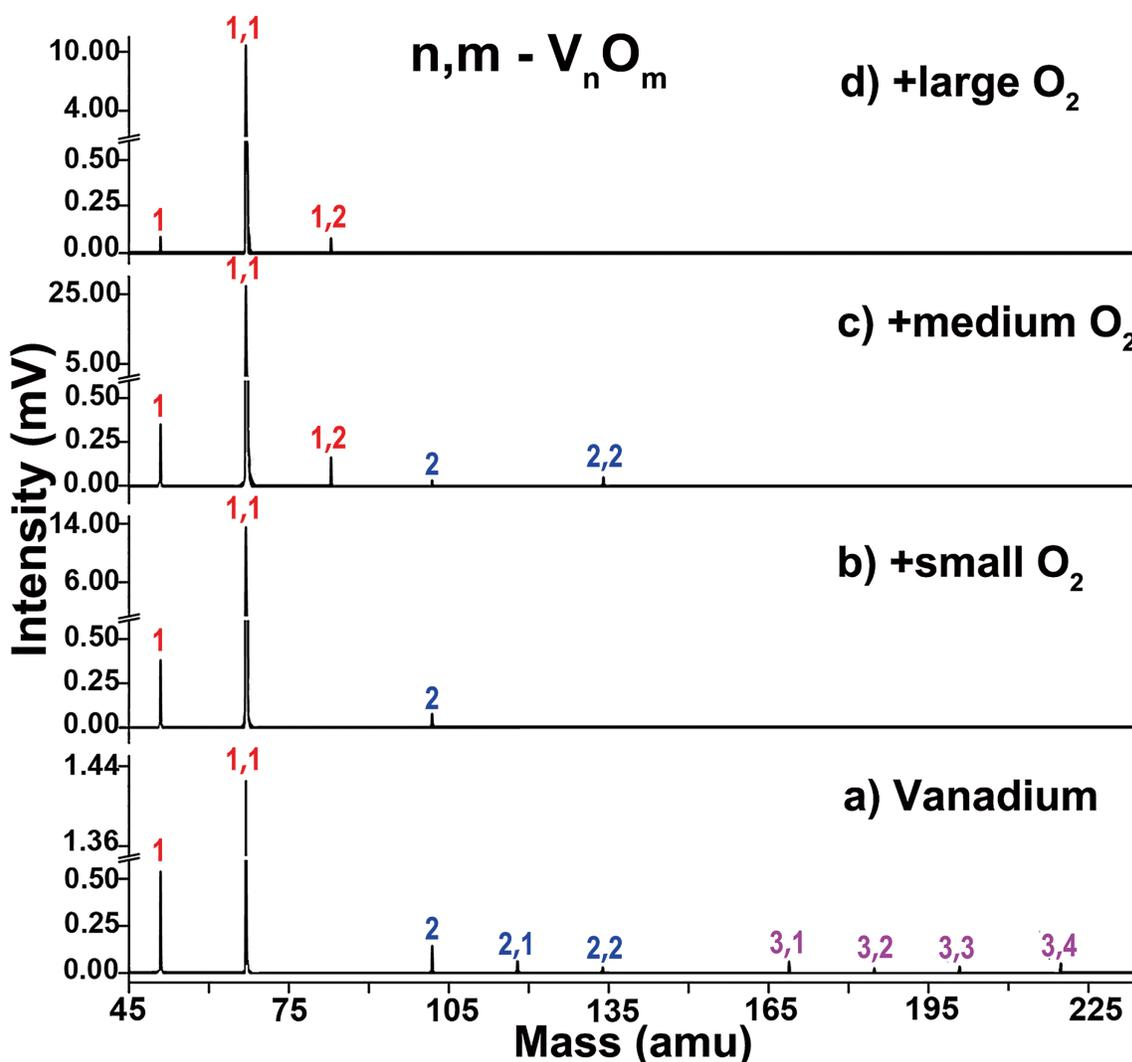
**Fig. S2** TOF mass spectra of small  $V_n$  ( $n=1-4$ ) clusters produced via a 1.0 cm nozzle at the absence (a) and presence (b-d) of oxygen added into the reaction tube. The amount of oxygen (0.1 MPa 3% $O_2$ /He) is controlled by the on-time width of pulsed valve: 200, 220, 250 $\mu$ s, respectively.
