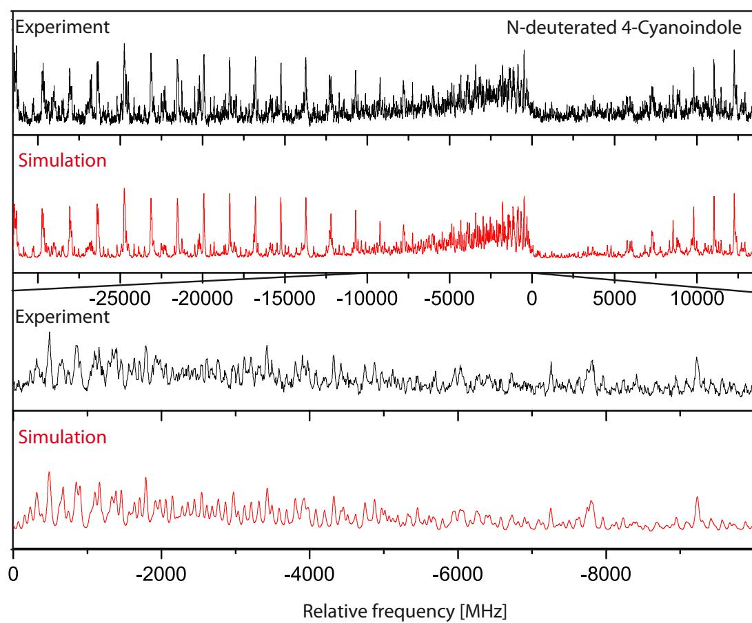
**Figure S4** Rotationally resolved electronic spectrum of the electronic origin of N-deuterated 4-cyanoindole
