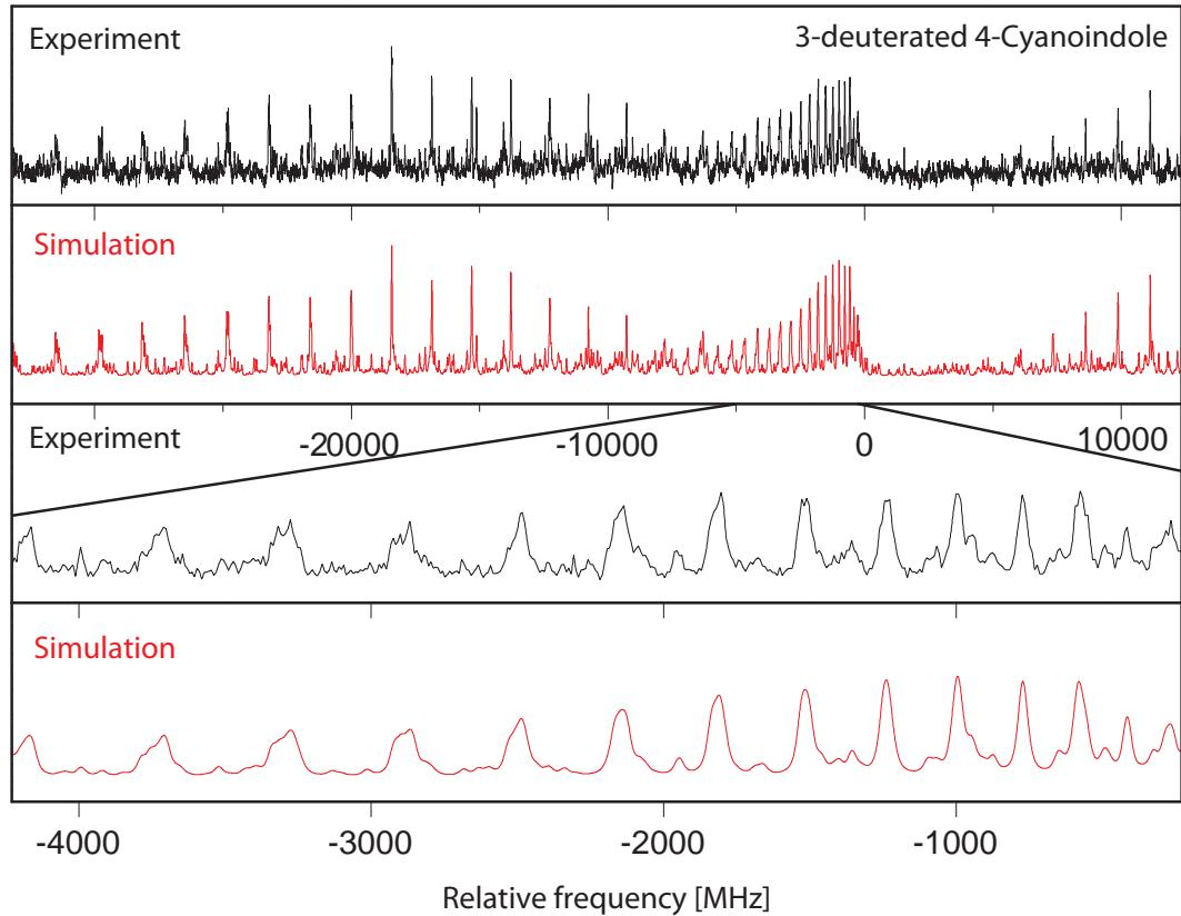
**Figure S6** Rotationally resolved electronic spectrum of the electronic origin of 3-deuterated 4-cyanoindole
