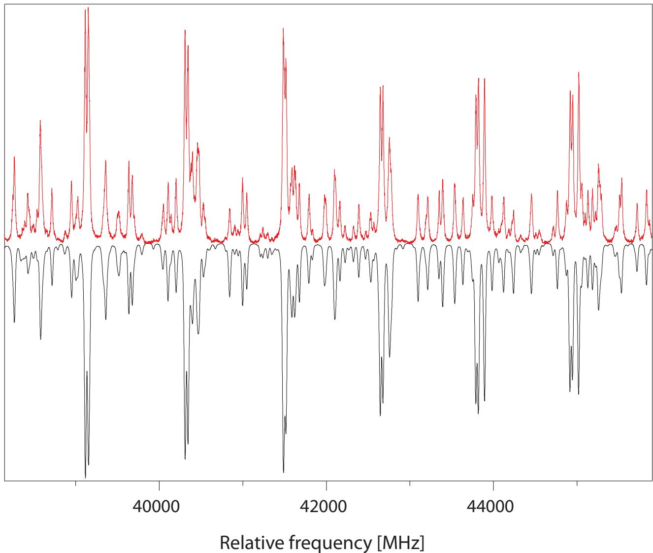
**Figure S3** Expanded view of the rotationally resolved electronic spectrum of the electronic origin of 4-cyanoindole along with a fit of the line form parameters to determine the fluorescence lifetime.
