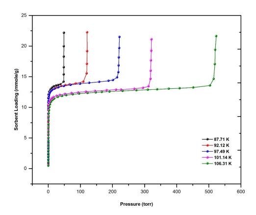
We determined the dose from a calibrated volume  $(V_{dose})$  and the difference between the initial and final pressure  $(P_i - P_f)$ . The amount  $(A_{vap})$  in the vapor phase inside the cell was determined from the final value of the pressure when equilibrium was reached and the effective value of the cell at the measured temperature. The amount adsorbed was the value of the sum total of gas added to the cell, minus the amount present in the vapor phase
