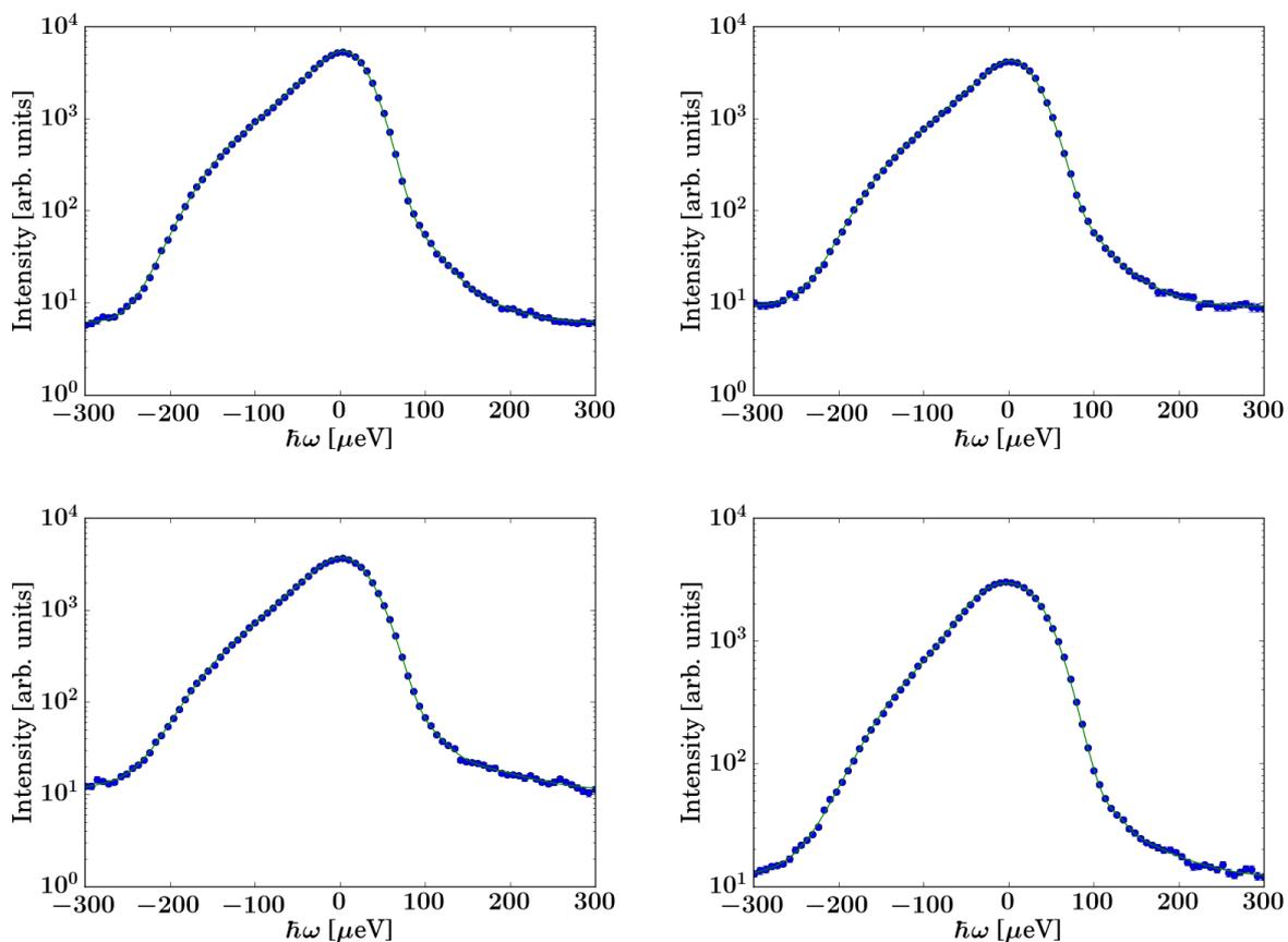
Figure S1: Energy resolution data of LET, measured on a frozen sample of 0.16 mole fraction ethanol in water ( $\text{H}_2\text{O}$ ) at  $T = 150 \text{ K}$  and  $3.4 \text{ meV}$  incident energy (symbols), and fits of a sum of 5 Gaussian functions and a constant base line (lines), at  $q = 0.55 \text{ \AA}^{-1}$  (top left),  $q = 1.05 \text{ \AA}^{-1}$  (top right),  $q = 1.55 \text{ \AA}^{-1}$  (bottom left), and  $q = 2.05 \text{ \AA}^{-1}$  (bottom right).
