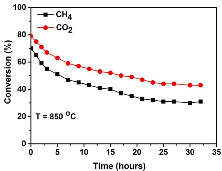
Figure S3: Time-on-stream stability test of  $\text{La}_{1.99}\text{Ru}_{0.01}\text{O}_3$  in a fixed-bed reactor at 850 °C for 32 h. Reaction conditions:  $\text{CO}_2/\text{CH}_4 = 1$ ,  $\text{CO}_2:\text{CH}_4:\text{N}_2 = 1:1:18$  (total flow rate = 20 sccm),  $\text{GHSV} = 20000 \text{ h}^{-1}$ .
