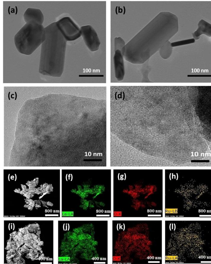
Figure S1: TEM images of as-synthesized (a-b)  $\text{La}_{1.99}\text{Ru}_{0.01}\text{O}_3$ . HR-TEM images of (c)  $\text{La}_{1.99}\text{Ru}_{0.01}\text{O}_3$  and (d)  $\text{La}_{1.98}\text{Ru}_{0.02}\text{O}_3$ . STEM-HAADF analyses are shown in (e-n).
