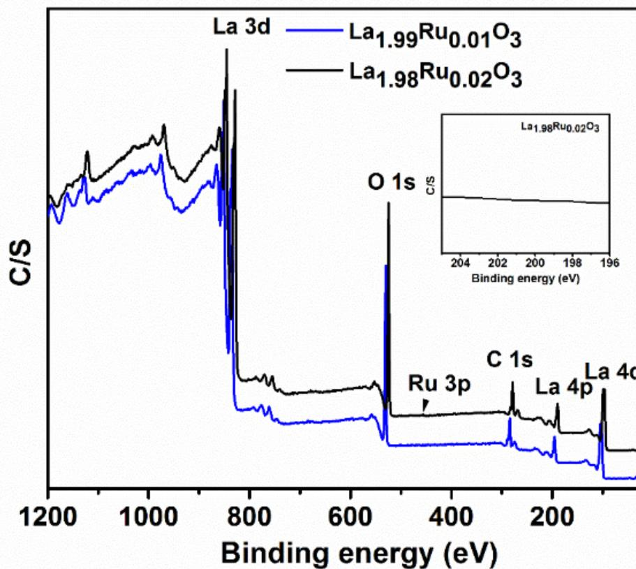
Figure S2: XPS survey scan for  $\text{La}_{1.99}\text{Ru}_{0.01}\text{O}_3$  and  $\text{La}_{1.98}\text{Ru}_{0.02}\text{O}_3$  catalysts. The inset image show expanded region for Cl(2p).
